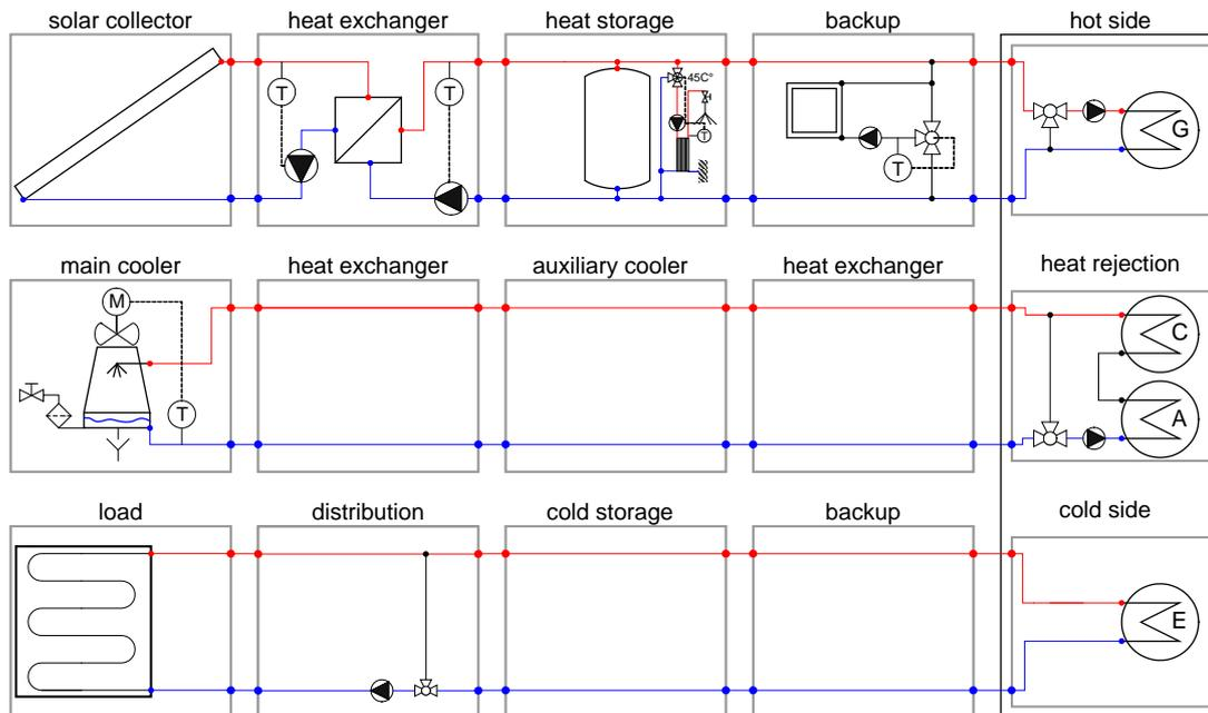
Fig. 4-5: Generic system: standardized system topology with placeholders for the integration of optional system components.
