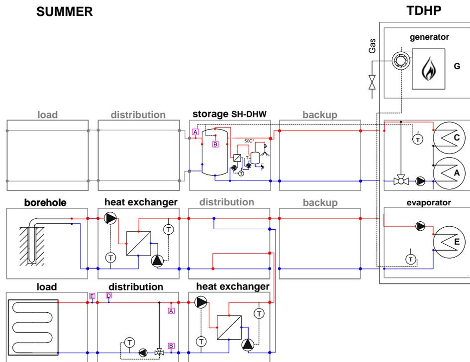
**Fig. 5-4:** Hydronic representation of a plant installed in the brewery’s storehouse in Graz
