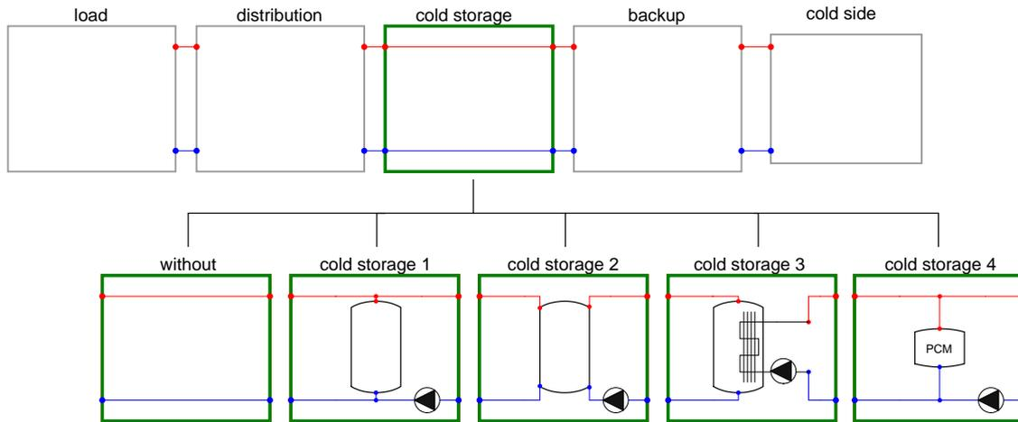
**Fig. 4-18: Chilled water sub-system: Chilled water storage and latent cold storage (PCM, phase change material).**
