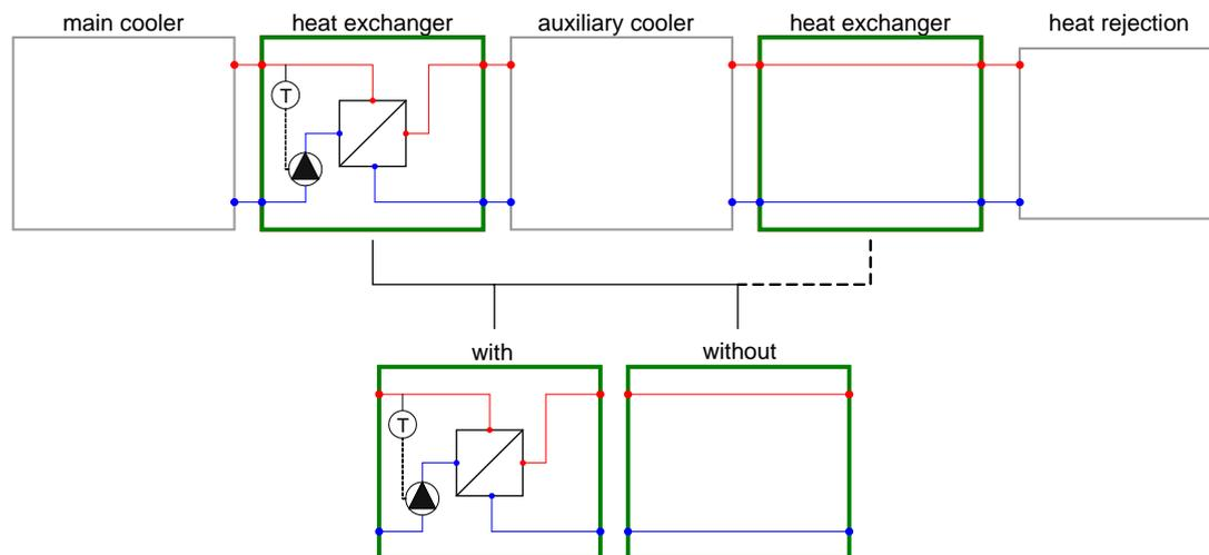
**Fig. 4-14: Heat rejection sub-system: optional heat exchangers for separation of thermally driven chiller, auxiliary cooler and main cooler.**
