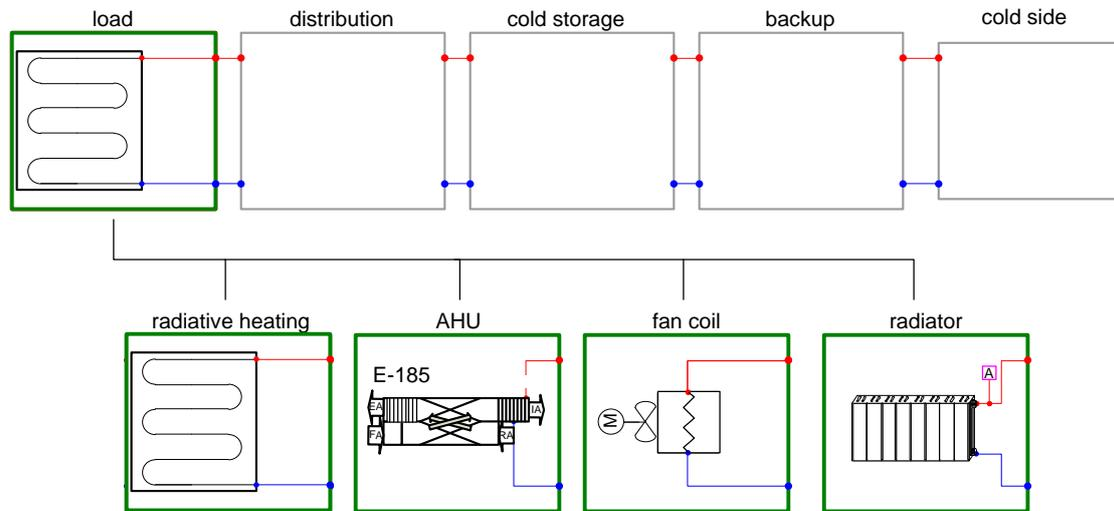
**Fig. 4-15: Heating appliances for utilization of the heat output of the sorption heat pump at intermediate temperature level for space heating.**
