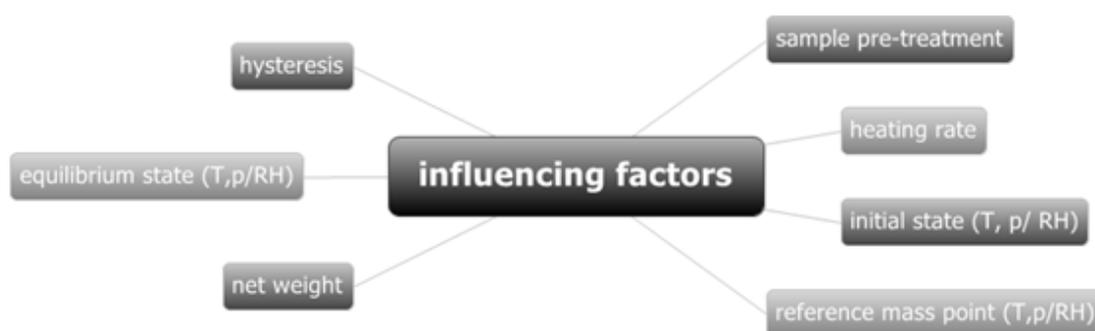
Fig. 3-11: Influencing factors for thermal analysis of the adsorption characteristics.
