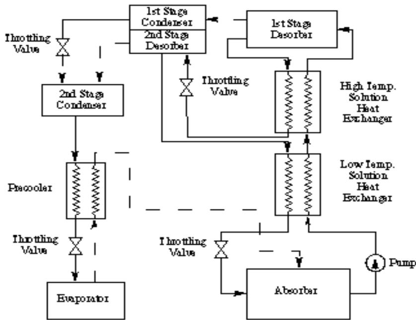
Fig. 1-10: Double effect absorption machine
