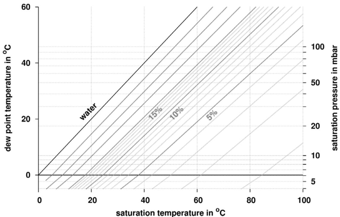
Fig. 1-18: Dühring-Diagram for Silica-Gel 127B. © Fraunhofer ISE
