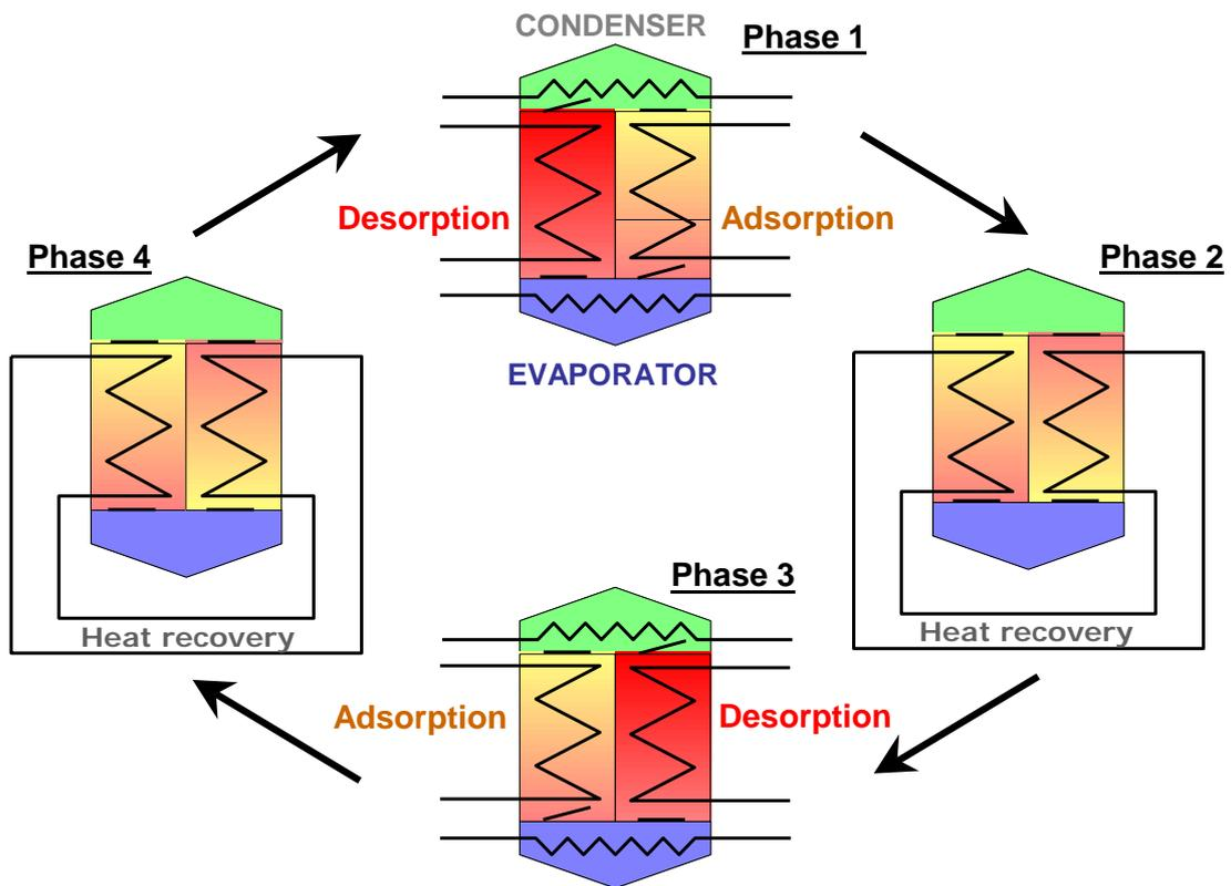
**Fig. 1-4: Simple adsorption schematic with heat recovery phase**
