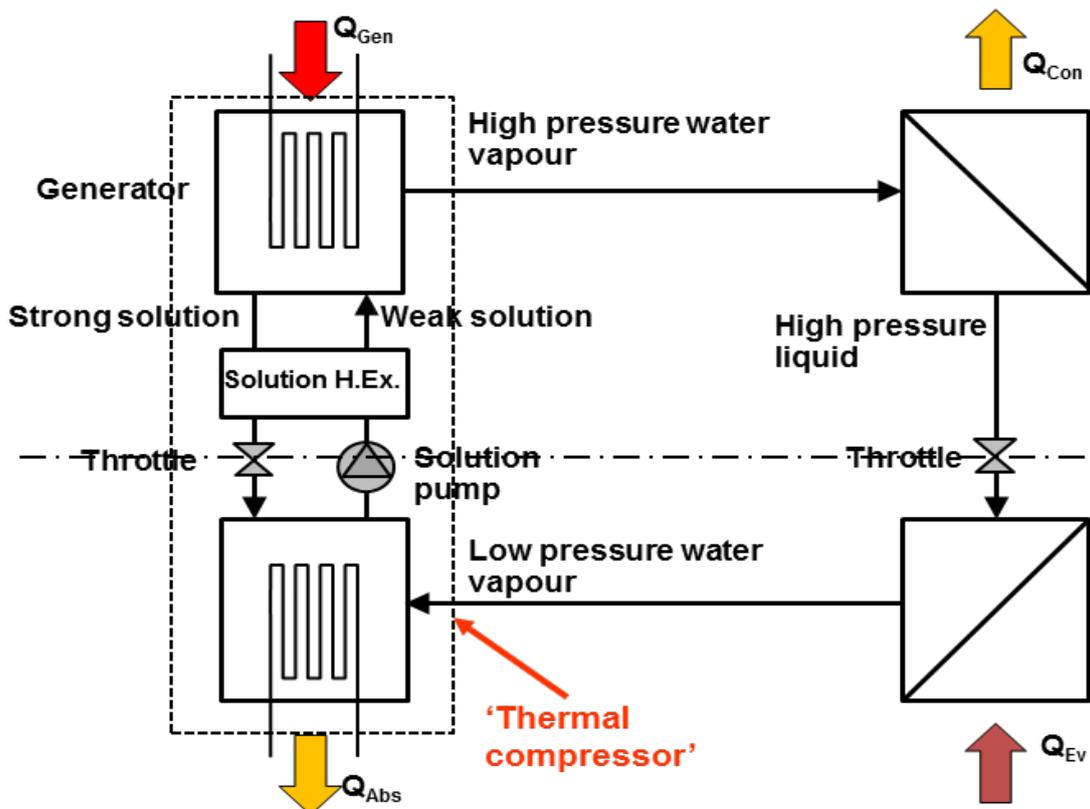
Fig. 1-3: Simple water - LiBr absorption cycle schematic
