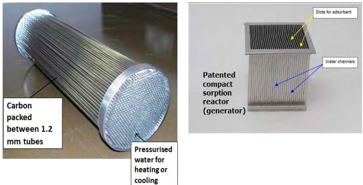
Fig. 1-8: Adsorbers developed at University of Warwick, UK
