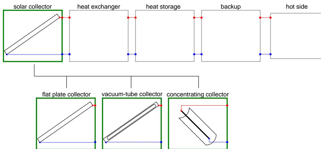
Fig. 4-7: Solar sub-system: options for the solar collector
