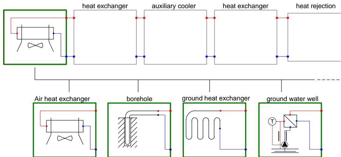
**Fig. 4-20: Heat sources for heat pump operation: Air-heat exchanger, boreholes geothermal collectors (ground heat exchanger) or ground water well,**
