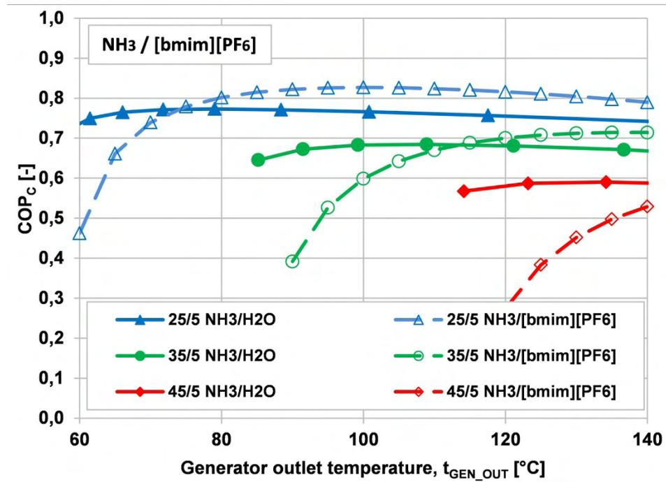
Fig. 3-22: Simulation results of the COP for  $t_{ABS}/t_{EVA}=25/5^\circ C$ ,  $35/5^\circ C$  and  $45/5^\circ C$  of  $NH_3/[bmim][PF_6]$  AHP-processes without rectification column in comparison to a conventional  $NH_3/H_2O$  AHP-process with rectification column depending on the generator outlet temperature
