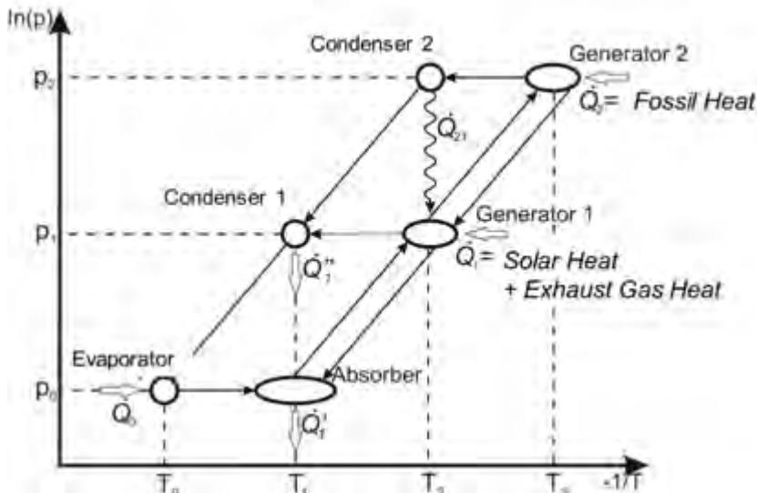
**Fig. 1-14: Double-/Single-effect absorption cycle in the  $\ln p/-1/T$ -diagram (Riepl, Gurtner et al. 2011)**
