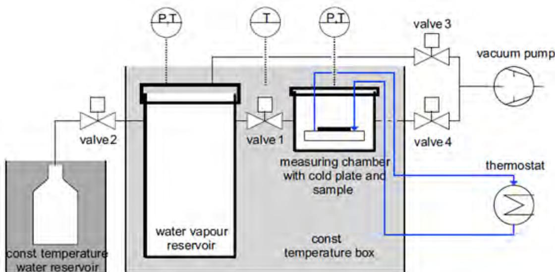
Fig. 3-4: Scheme of the entire kinetic measurement setup.
