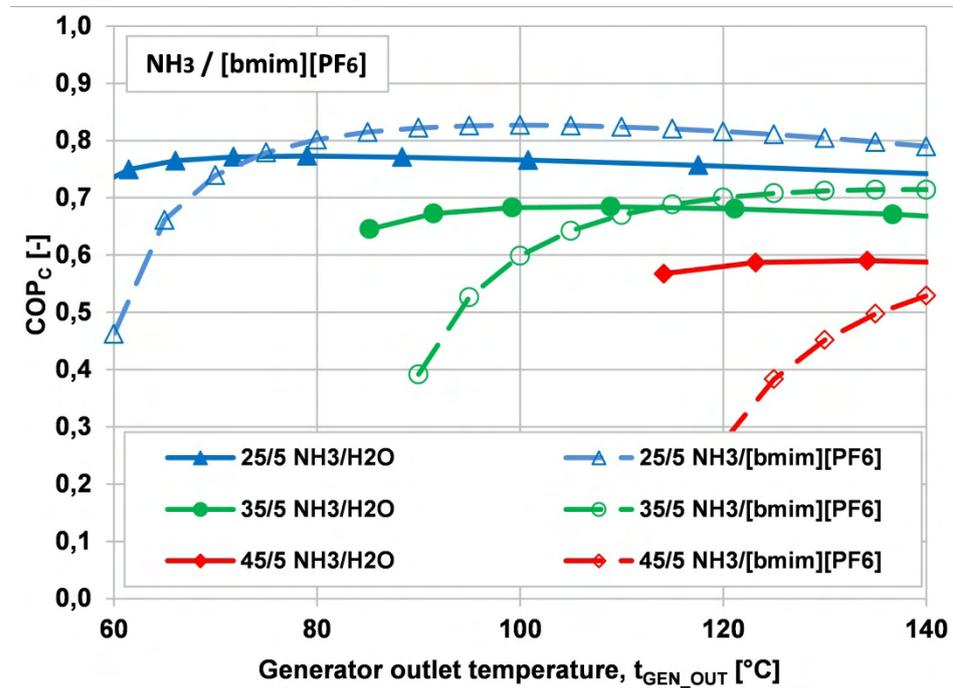
Fig. 3-22: Simulation results of the COP for  $t_{ABS}/t_{EVA}=25/5^\circ C$ ,  $35/5^\circ C$  and  $45/5^\circ C$  of  $NH_3/[bmim][PF_6]$  AHP-processes without rectification column in comparison to a conventional  $NH_3/H_2O$  AHP-process with rectification column depending on the generator outlet temperature
