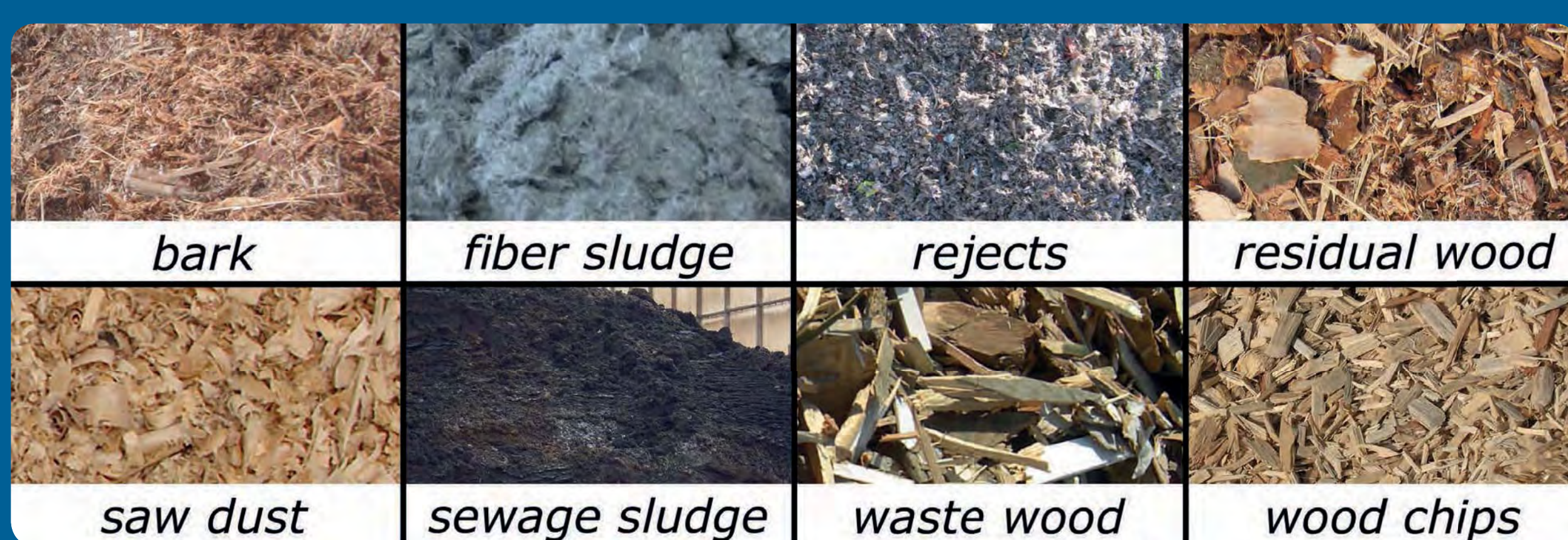
Figure 2: Biomass and biomass waste fuels utilized by Austrian fluidized bed plants
