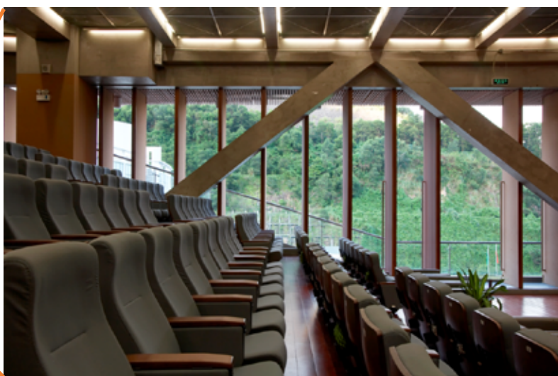
A typical mixed-mode building. The auditorium was designed with openable walls to make good use of natural ventilation. This space has achieved good thermal comfort and low energy consumption. Source: Shenzhen iBR, P.R. China
