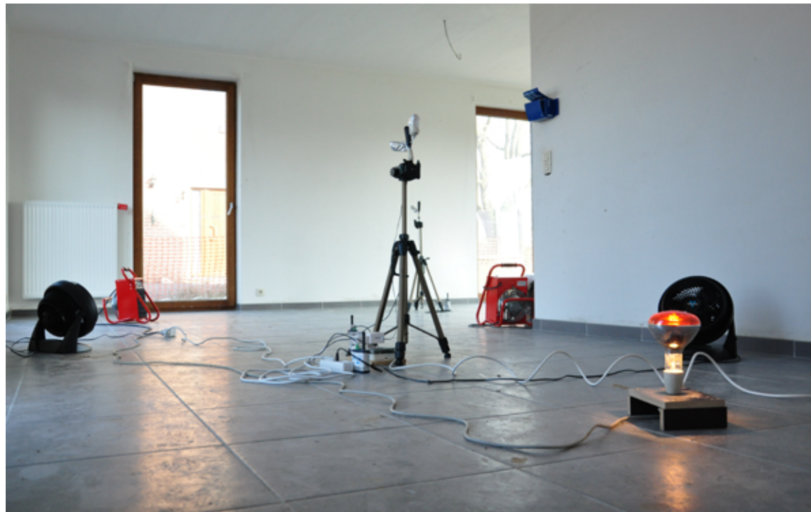
On site building fabric performance assessment by a co-heating test. By measuring the heat input necessary to heat the dwelling to an elevated steady-state temperature, the overall actual heat loss coefficient can be determined and compared with the design value.
