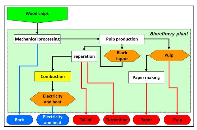
**Figure 11:** 3-platform (black liquor, pulp, electricity&heat) biorefinery using wood chips for pulp, paper, turpentine, tall oil, bark, electricity and heat
