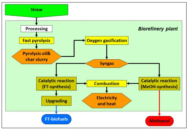
**Figure 71:** 3-platform (pyrolysis oil, syngas, electricity&heat) biorefinery using straw for FT-biofuels and methanol with oxygen gasification
