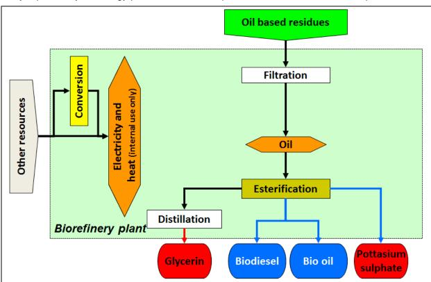
Figure 51: 1-platform (oil) biorefinery using oil based residues for biodiesel, glycerine, bio oil and fertilizer
