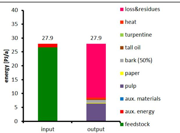
Figure 13: Energy balance of biorefinery plant
