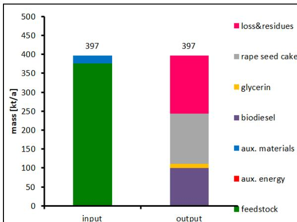
Figure 42: Mass balance of biorefinery plant
