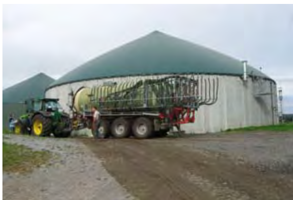
Photo 4: Digestate being taken from a digestate tank by a tractor and slurry tanker
