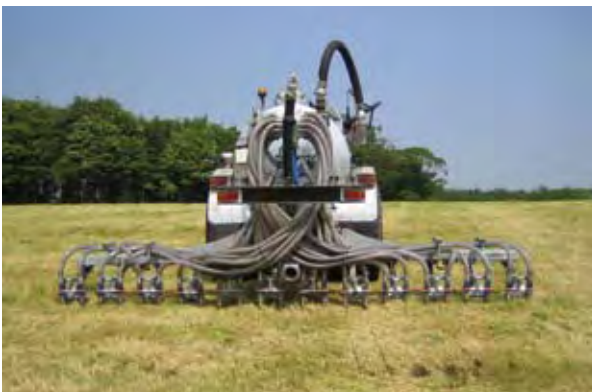
Photo 6: Trailing-shoe application places digestate on the soil surface beneath any foliage
