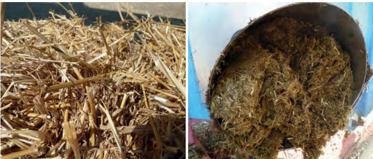
Figure 10: Unextruded (left) and extruded (right) wheat straw (photo by Ludek Kamarad).
