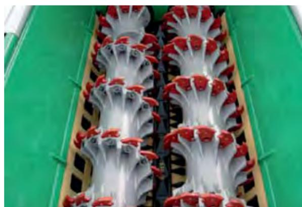
Figure 5: Example of a shredder called CRAMBO by Komptech GmbH, Austria (image from Komptech).
