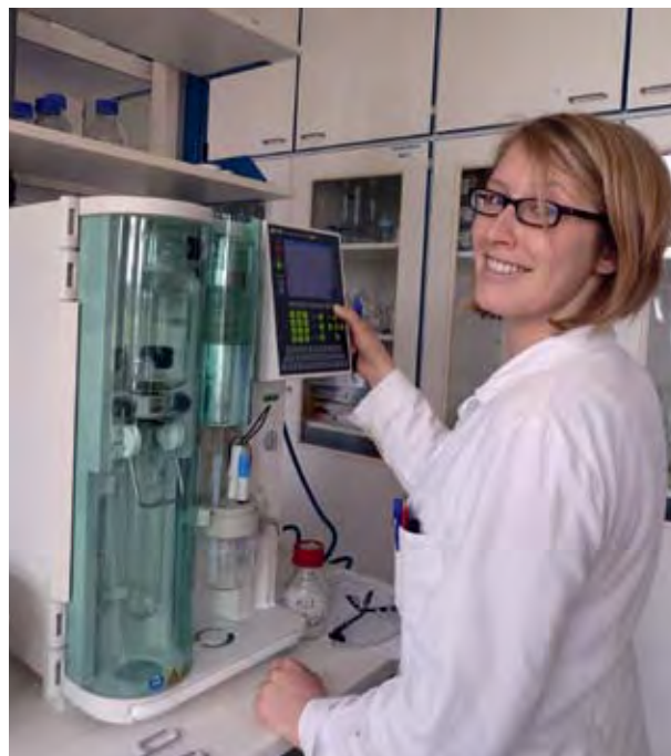
Figure 10 Automated distillation laboratory system for measuring ammonium nitrogen (NH 4 -N), Total Kjeldahl nitrogen (TKN) can also be determined after a sample pre-treatment (© Markus Ortner, IFA Tulln)
