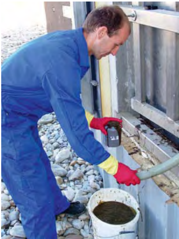
Figure 17 Sampling of the digester content at a biogas plant. At the sampling valve the first output of the digester is discharged and then the sample is taken. Adequate clothing and gloves should be used during sampling (© IFA Tulln).
