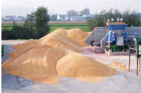
Photo 8: Solid substrate grinder (right) as used for preparation of the dry substrates (maize) in anaerobic digestion of crops
