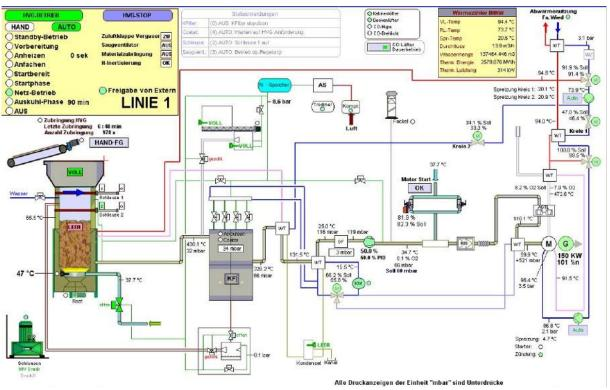
**Figure 6: Flow sheet – Urbas gasifiers**
