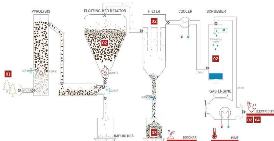
**Figure 8: SynCraft technology – flow sheet**
