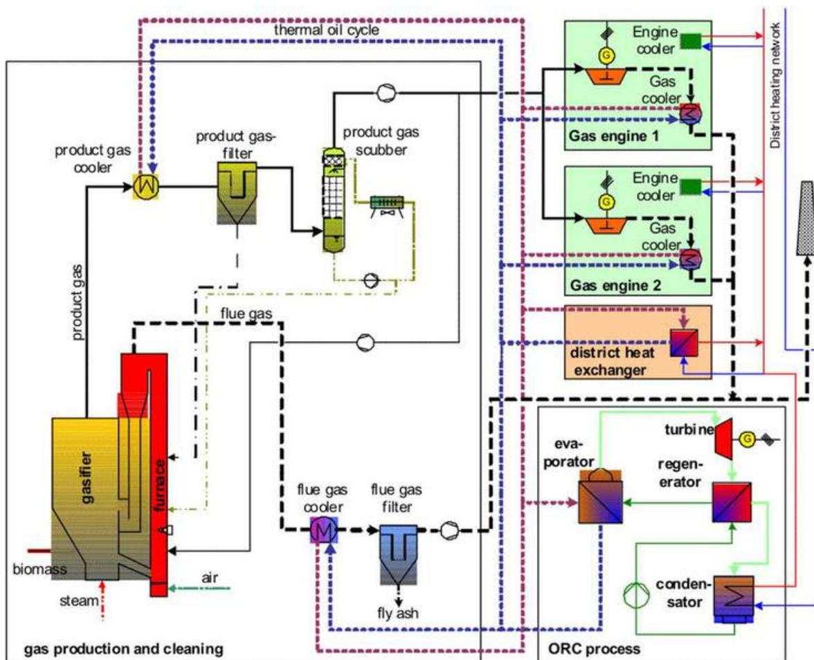
Figure 5: FICFB plant with ORC - flow sheet
