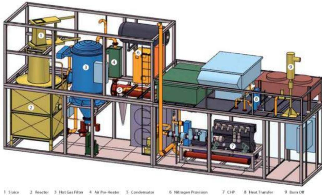
**Fig. 7: Urbas gasifier – container type**
