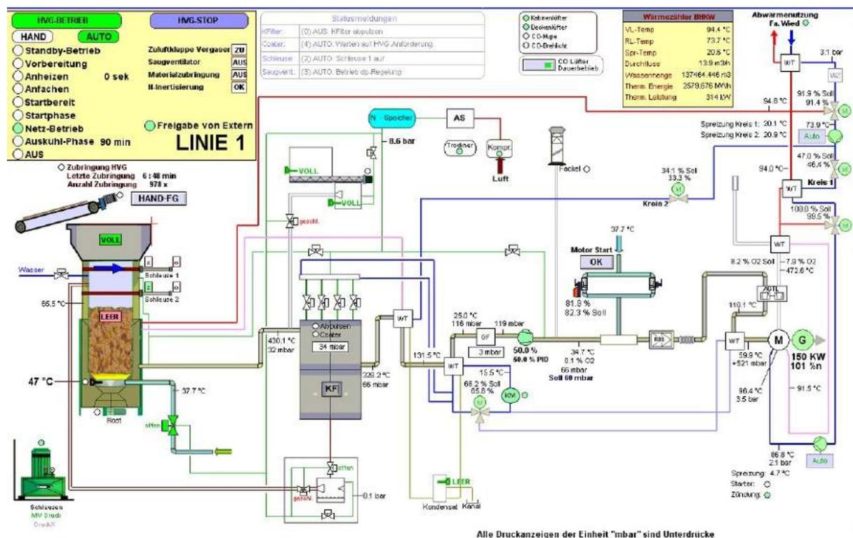
Figure 6: Flow sheet – Urbas gasifiers
