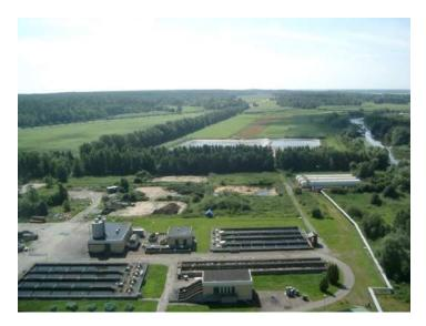
Figure 5.14. View of a municipal wastewater plant in Enköping, Sweden, with water storage ponds and (behind the ponds) the willow fields that are used as vegetation filters. The photo is taken from the roof of the heat and power plant that uses the locally produced biomass (Photo: Pär Aronsson, SLU).
