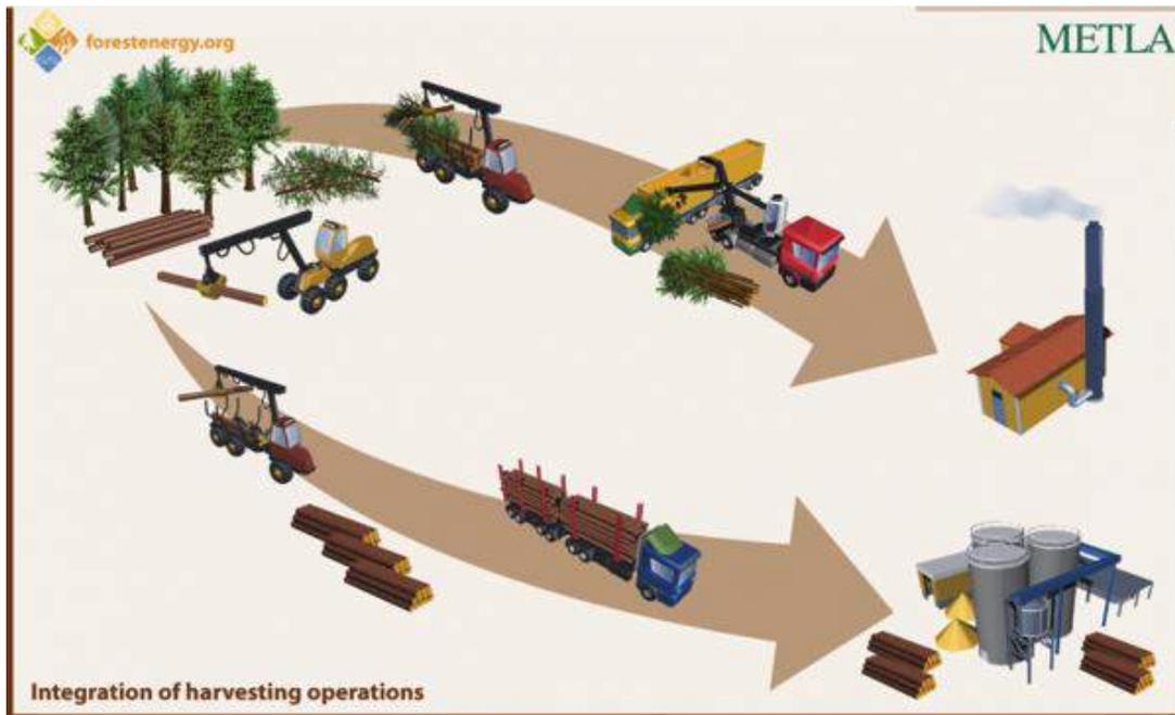
Figure 2.6. Integrated harvesting and transport of residual forest biomass and roundwood supply.
