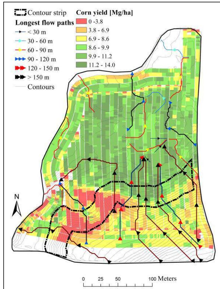
Figure 5.13. Final design of the contour buffer.
