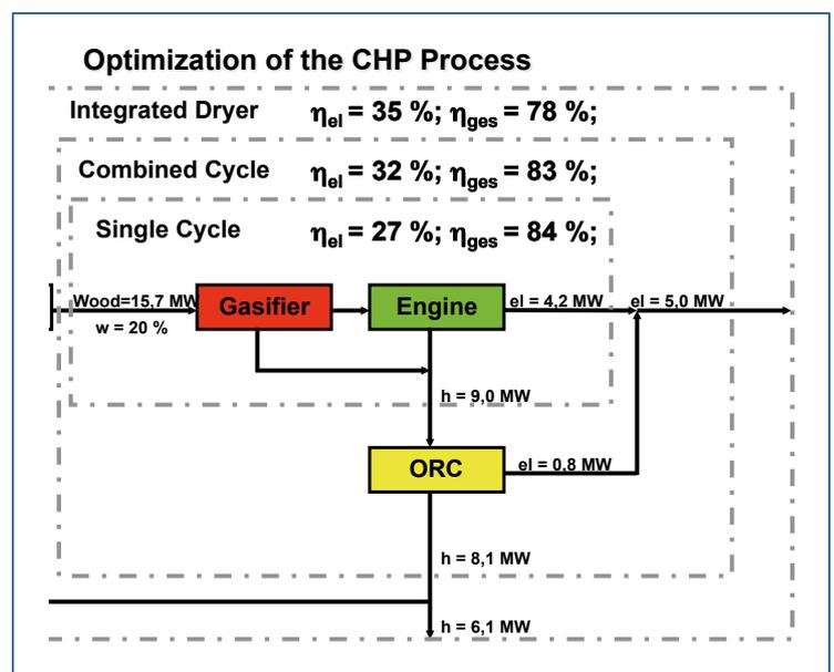
**Figure 15:** Measures to increase the total efficiency of the CHP process
