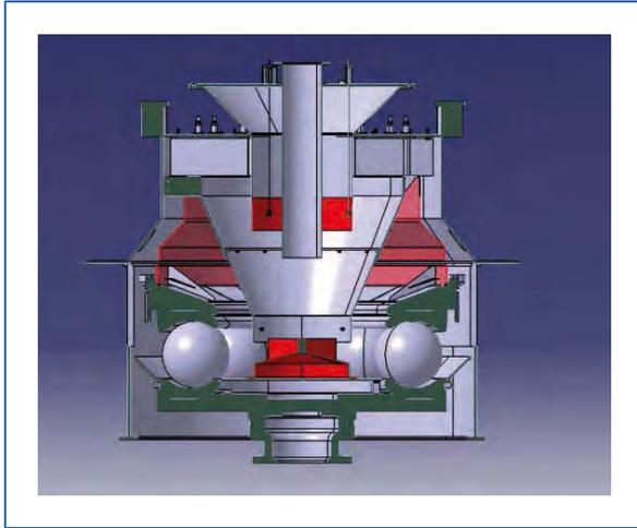
**Figure 19:** Ball and ring mill modified for processing wood pellets
