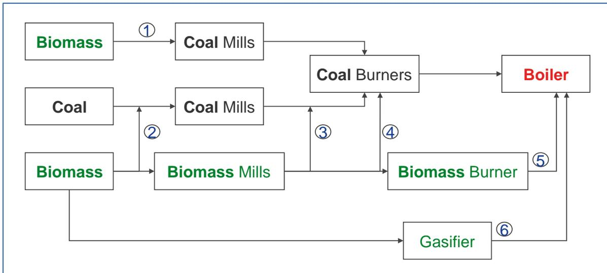
**Figure 18:** The principal direct and indirect biomass co-firing options
