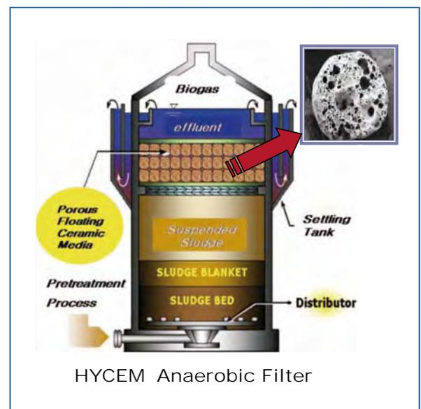
**Figure 13:** Digestion of the liquid part of separated manure in a hybrid filter
