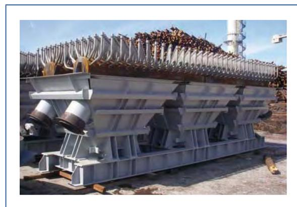
**Figure 9:** Bubbling Fluidised Bed technology before integration into an existing boiler
