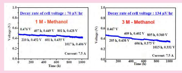
Figure 23 Operating over 1000hrs, and utilising concentrations of methanol at 1M and 3M, the above figures demonstrate the increased aging of the cell that is operated with the higher methanol concentration
