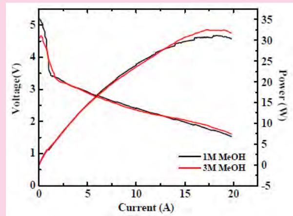
**Figure 23 Operating over 1000hrs, and utilising concentrations of methanol at 1M and 3M, the above figures demonstrate the increased aging of the cell that is operated with the higher methanol concentration**
