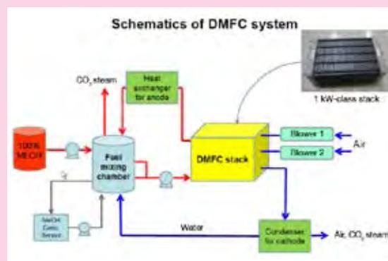
A power pack for military use has been developed by a consortium at KIER, Chungnam Nat'l University and KAIST in Korea. The power pack weighs 1.2 kg and provides 24 W of portable power, 30 W at peak power, and operates between 32-65 °C for 500 hours. This has been developed as a concept product to directly replace batteries so that the challenge of recharging time is removed as well as offering low temperature operation, a quiet product and a high efficiency system.
