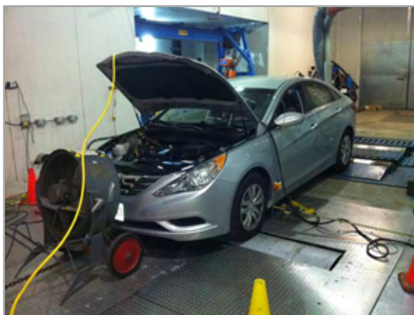
Fig. 1 Vehicle Emissions Testing on Environment Canada's Chassis Dynamometer
