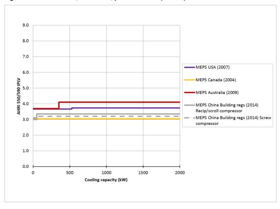
Figure 9. MEPS chillers, air-cooled, part load IPLV (kW/kW).
