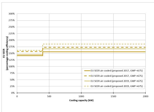
Figure 10. Proposed MEPS for EU chillers, air-cooled, seasonal efficiency SEER (expressed as percentage useful cooling efficiency). GWP is the global warming potential of the refrigerant used in the chiller.
