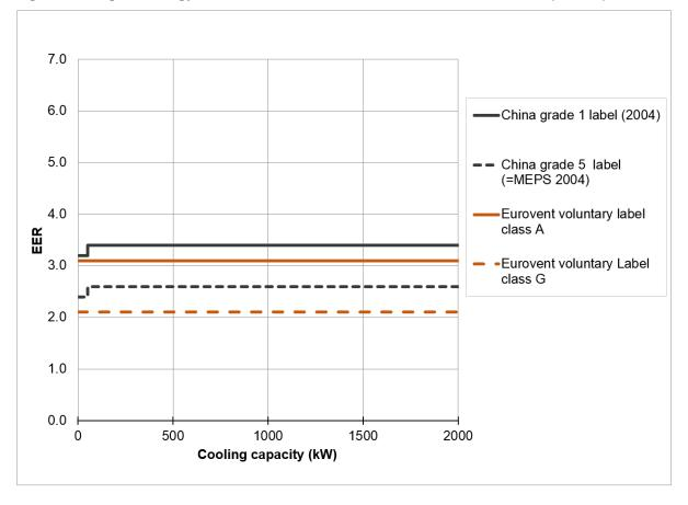
Figure 8. Range of energy labels for air-cooled chillers, full load EER or COP (kW/kW).
