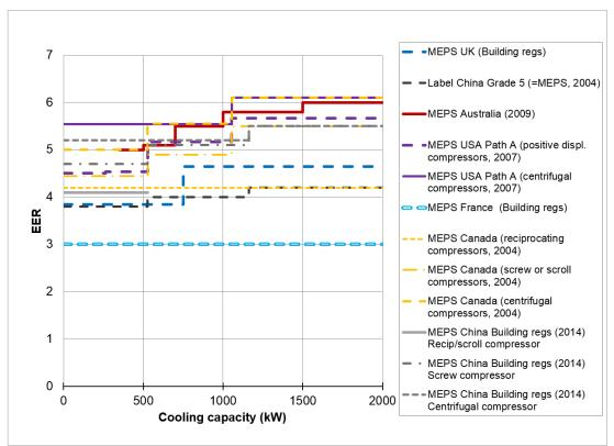
Figure S2. Comparing existing MEPS for water-cooled chillers for comfort cooling applications that are based on full load efficiency (COP or EER).
