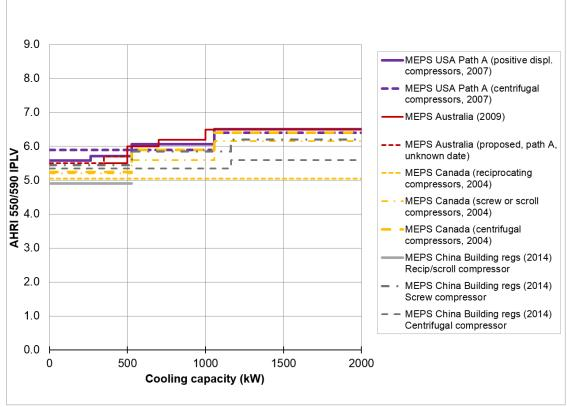
Figure 13. MEPS for water-cooled chillers, part load IPLV, general and 'Path A' (kW/kW).
