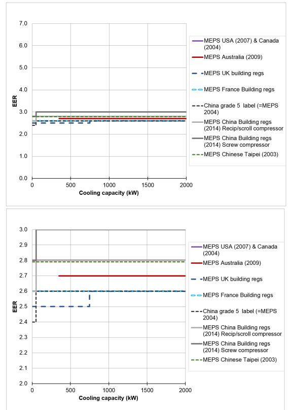
Figure 7. MEPS chillers, air-cooled, full load EER (kW/kW). Upper graph is set for direct comparison with Figure 11 and Figure 12; the same data appears in lower graph, but zoomed in for clarity.
