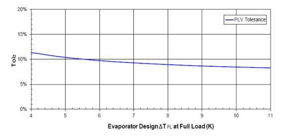
The water temperature difference across the evaporator is around 5K. This leads to a tolerance level close to 10.5%.
