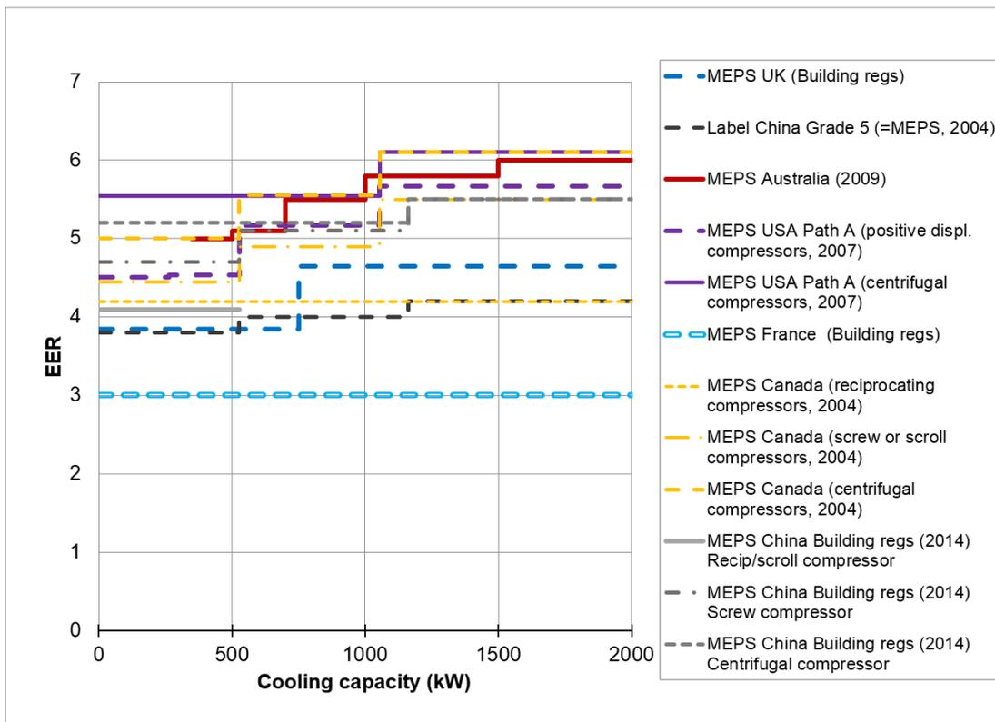
**Figure 12. MEPS for water-cooled chillers, full load EER, general and 'Path B' for comfort cooling applications (kW/kW).**
