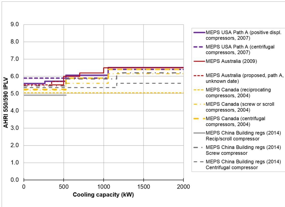
**Figure 14. MEPS for water-cooled chillers, part load IPLV, general and 'Path B' (kW/kW).**
