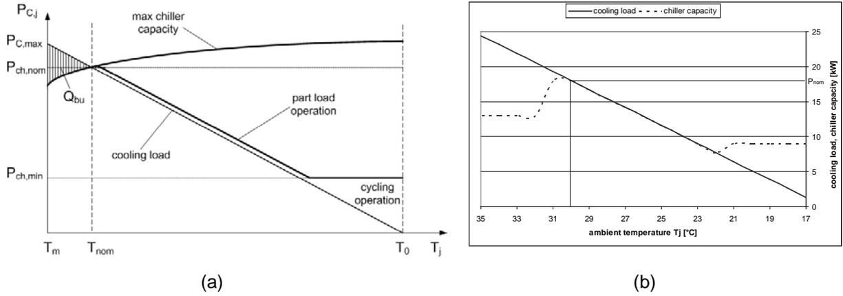
Figure 3: Approximation of the cooling load for given climate and nominal chilling power in theory (a) and calculated from assumed data and climate conditions with the proposed method (b)
