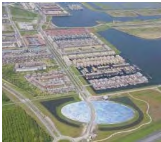
▲ Solar Island in Almere with 7,000 m 2 of solar collectors was the first solar district heating system in The Netherlands.
