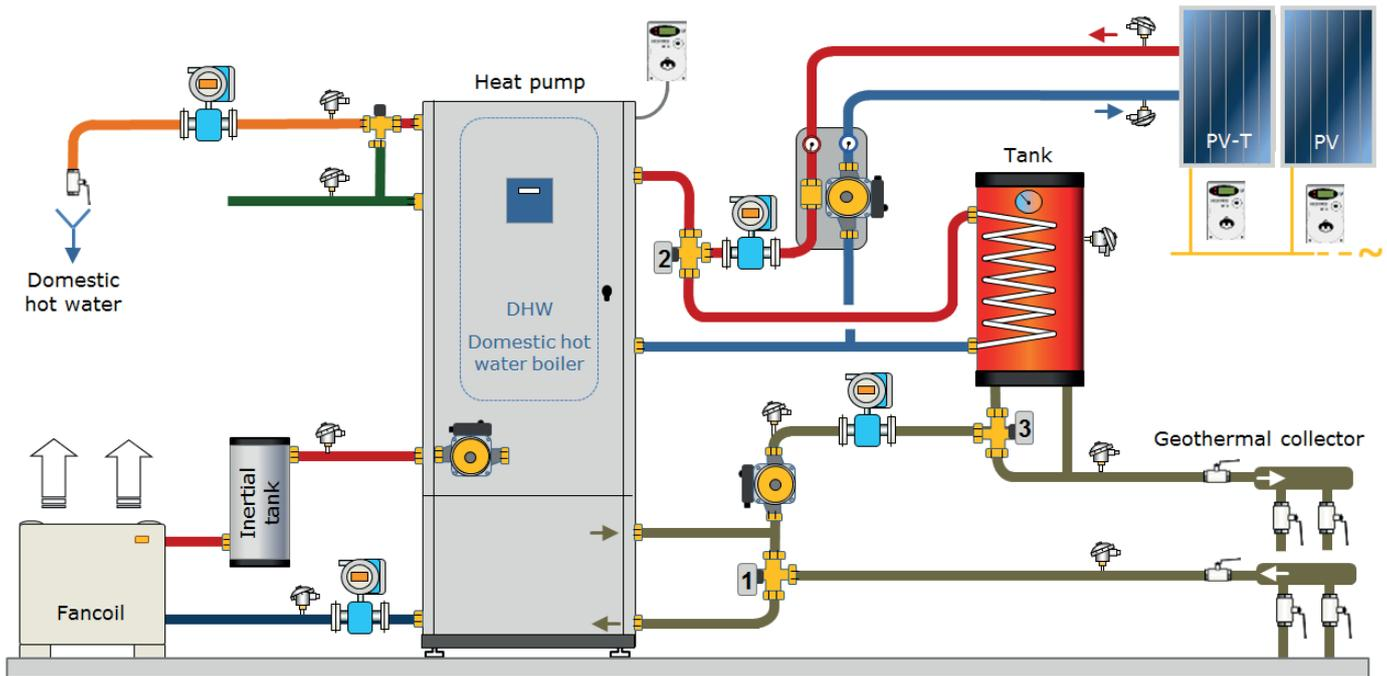
Figure 2. Plant scheme and monitoring system
