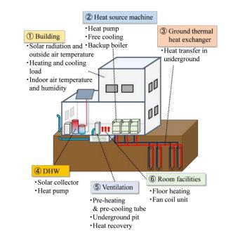
Figure 5. Structure of the ZEB simulator
