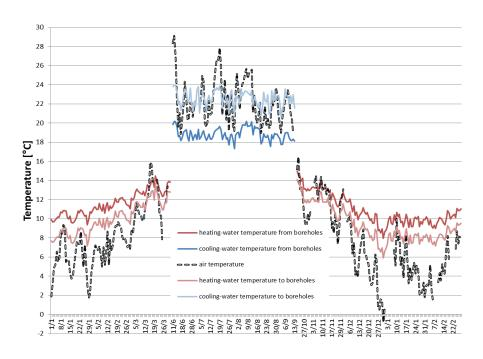
Figure 3. Daily average temperature of external air and of water from boreholes
