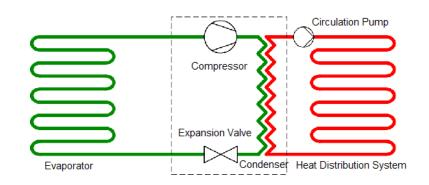
Figure 3. Direct Exchange Ground Coupled System
