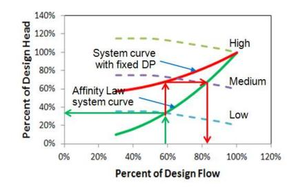
*Figure 3. Conventional pumping control with fixed differential pressure set point results in overflow at part load conditions*
