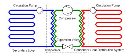
Figure 2. Secondary Loop Ground-Coupled System
