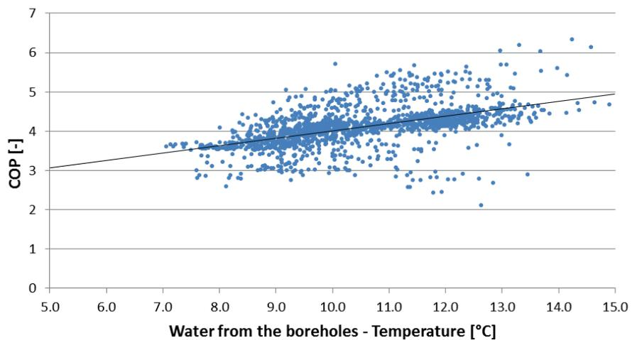
Figure 4. Hourly average COP related to hourly average water temperature from boreholes
