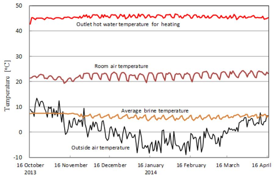
Figure 3. GSHP heating system for the primary school building in Kuromatsunai town
