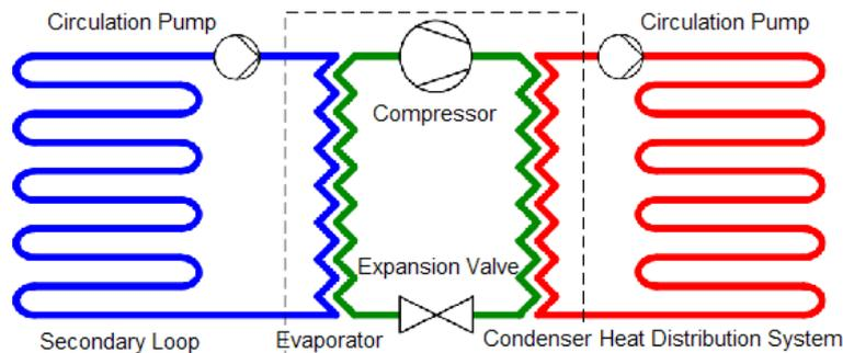
Figure 2. Secondary Loop Ground-Coupled System
