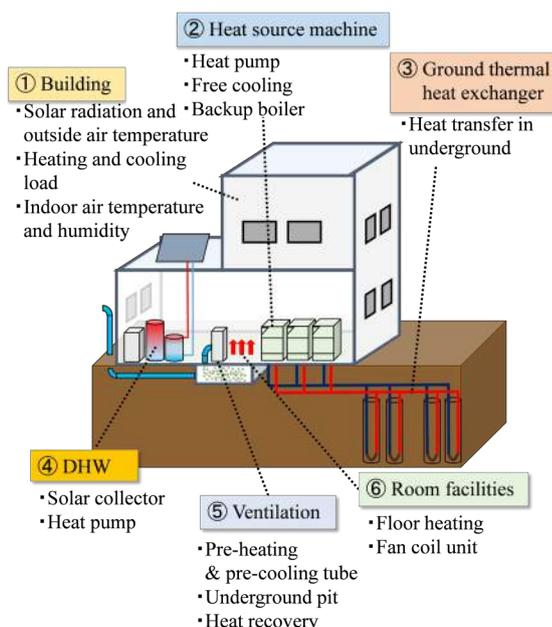
Figure 5. Structure of the ZEB simulator
