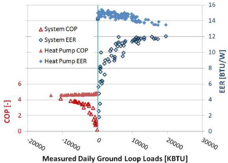
Figure 2. GSHP system efficiency vs. heat pump efficiency at various loading conditions (example results of case # 2)
