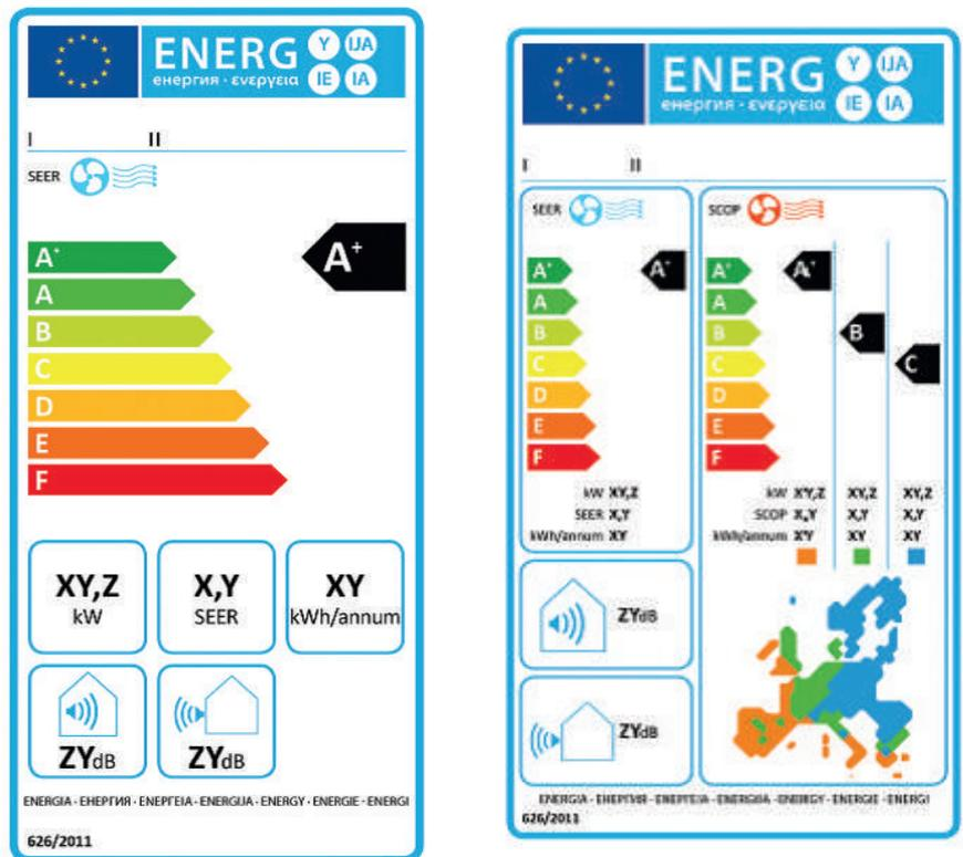
Figure 1. Energy labelling of air-to-air conditioners < 12 kW - Labels as applicable from 1<sup>st</sup> January 2015 (left hand side: cooling only units – right hand side: reversible units)
