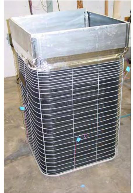
Figure 2. ASHP test unit in chamber – outdoor section
