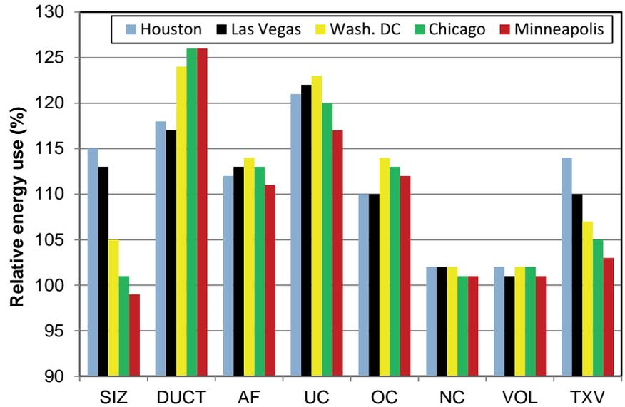
Figure 2. Annual energy use by a heat pump in a slab-on-grade house resulting from a single-fault installation, referenced to a fault-free installation. Fault levels: SIZ +50%, DUCT +30%, AF -36%, UC -30%, OC +30%, NC +10%, VOL +8%, and TXV -40%. (NIST contribution)
