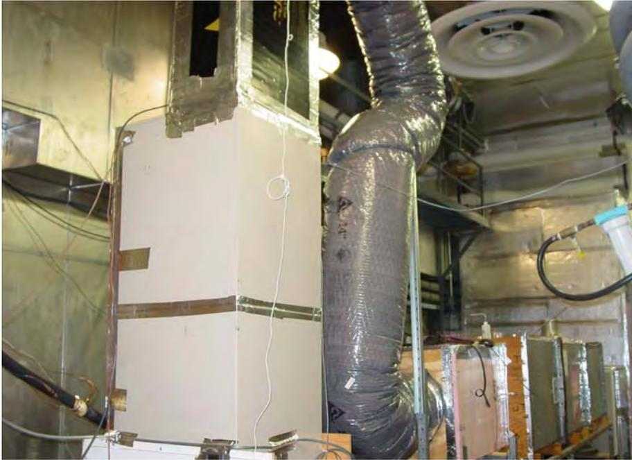
Figure 1. ASHP test unit in chamber – indoor section
