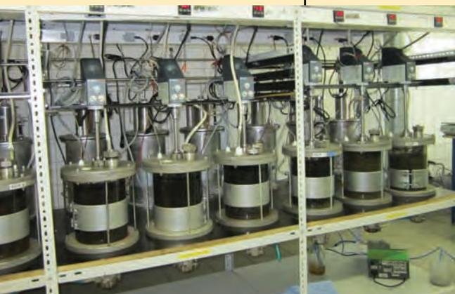
Two stage fermentation testing of biogas feedstocks at IFA Tulln.
