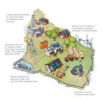
Figure 1: Systems architecture of EcoGrid EU in Bornhom
