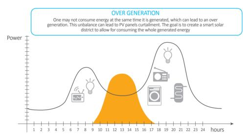
Figure 5: Illustration of the difference that can be noticed between the photovoltaic power gen eration curve and the consumer's power consumption
