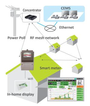
Figure 2: Smart meter system configuration
