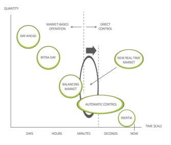
Figure 3: The new EcoGrid EU real-time market in the context of existing power balancing markets and control systems
