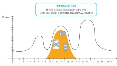
Figure 6: Illustration of the possible shift of a part of consumer's consumption to the periods when a surplus photovoltaic power is generated locally
