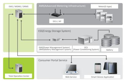
Figure 2: Key smart grid devices deployed for DSM
