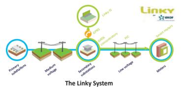
Figure 3: The Linky system, the basic building block of NICE GRID
