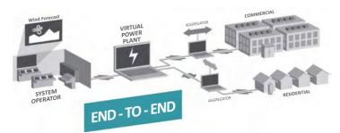
Figure 2: High-level system architecture for PowerShift Atlantic virtual power plants
