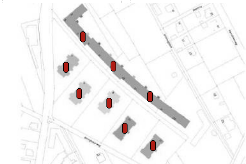
Figure 15: Site plan showing the position of the heat storage tanks. [Source site-plan: Hohensinn ZT GmbH]
