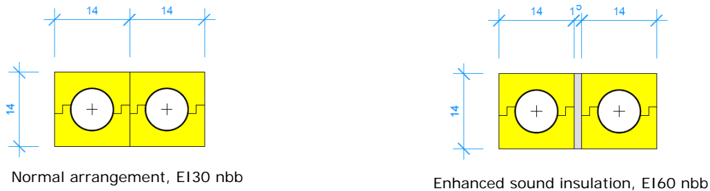
Figure 31: Sound control between parallel ventilation ducts
