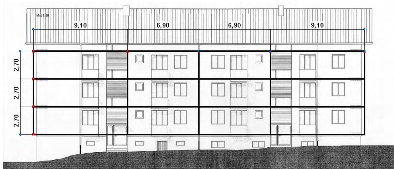
Figure 6: Possible façade subdivision into large-size units with maximum size of 10 m x 3.5 m
