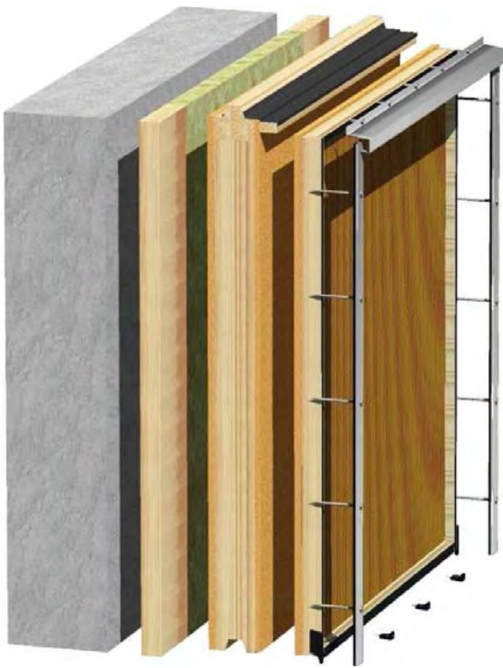
Figure 4: Layer composition of the basic façade module (Source: gap-solution GmbH)
