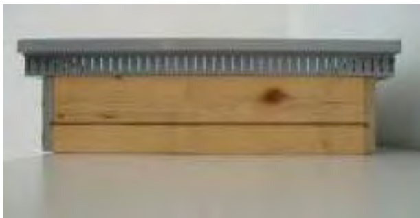
Figure 22: The prototype of the façade module. The timber frame and the ventilation slots can be seen. (Source: gap-solution GmbH)
