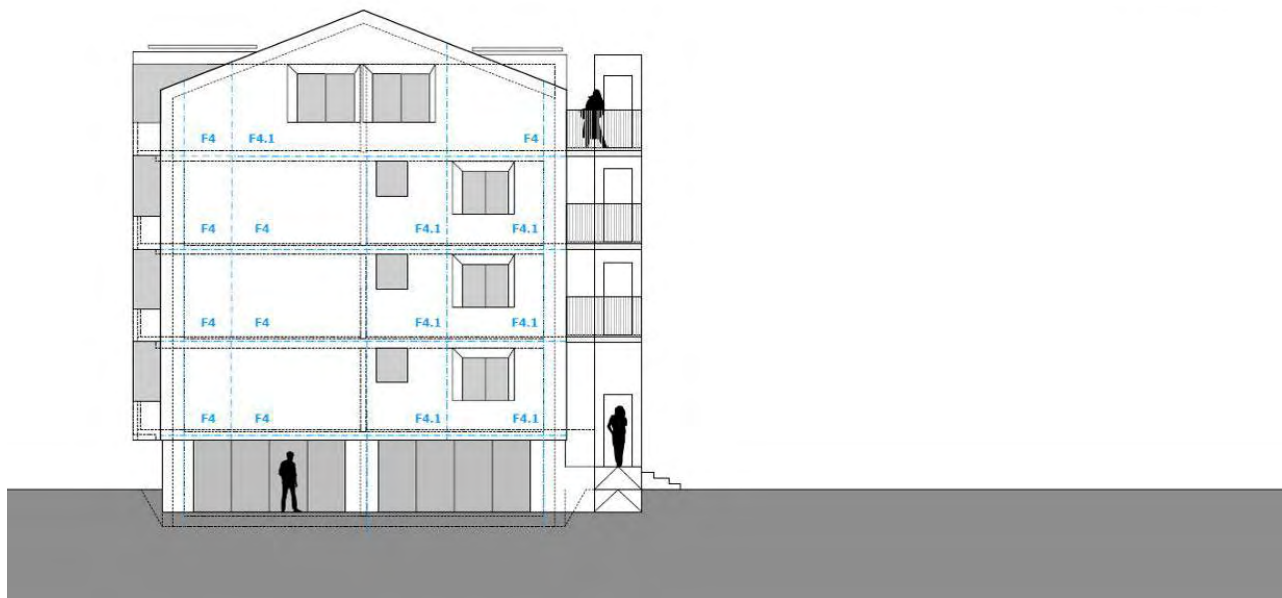
Figure 11: Southeast elevation (street-side façade with new office rooms in place of garages)
