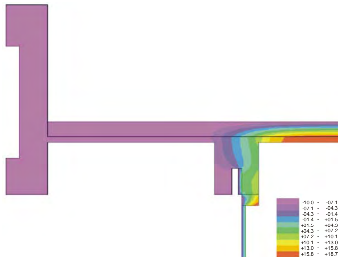
Figure 3: Typical thermal bridge of a projecting roof with an concrete attic
