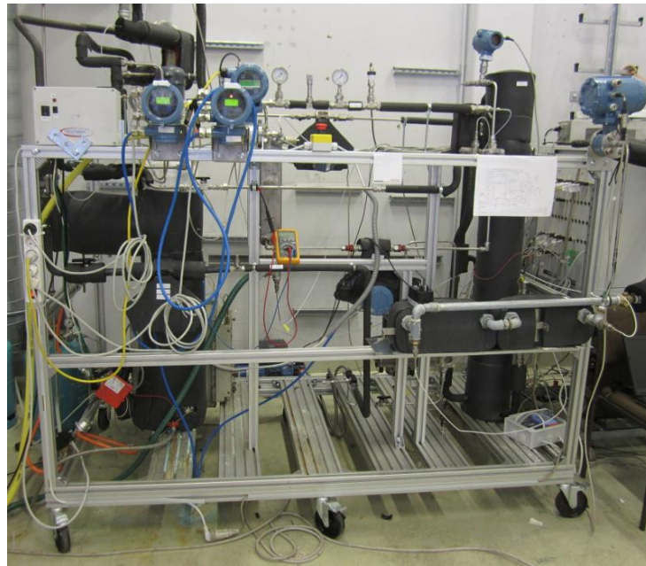
Figure 21: A combined generator-absorber set-up to verify the simulations in the NexGen Project.
