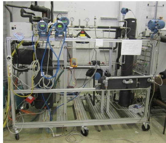
Figure 40: A combined generator-absorber set-up to verify the simulations in the NexGen Project.
