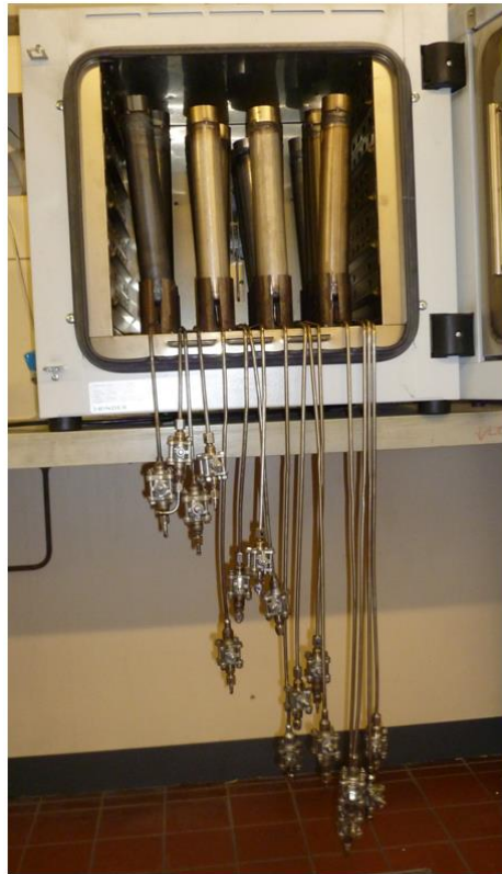
Figure 44: Autoclaves in the oven (Rieberer 2013)
