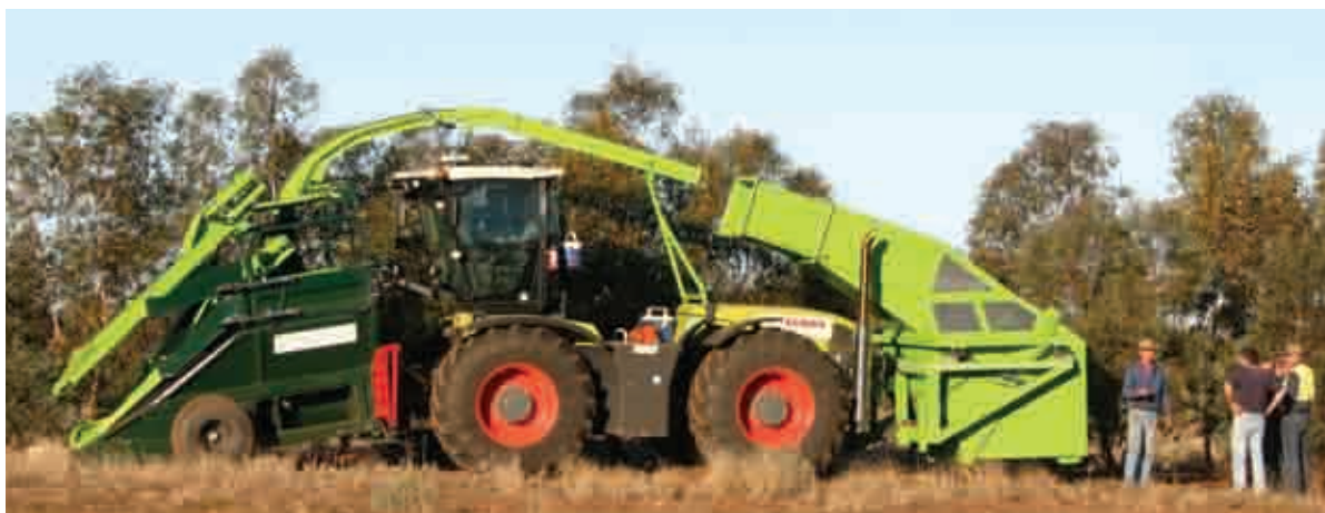
Figure 18. Mallee Eucalypt Harvester. Courtesy Rick Giles, DEC; Richard Sulman, Biosystems Engineering, and The Future Farm Industries Cooperative Research Centre.
