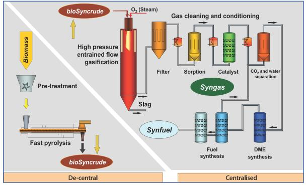
Figure 7. Schematic layout of the Bioliq process.
