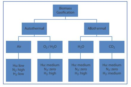
Figure 9. The different gasification systems.
