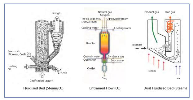
Figure 12. Basic designs of fluidised bed and entrained flow reactors.
