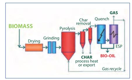
Figure 5. Elements of fast pyrolysis systems.
