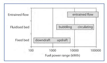
Figure 10. Typical gasifier designs by thermal power function.
