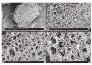
Photo 1. Typical molecular sieve structure of a carefully produced biochar.
