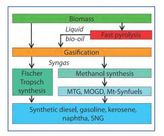
Figure 6. Possible processes from biomass to (liquid) biofuel.
