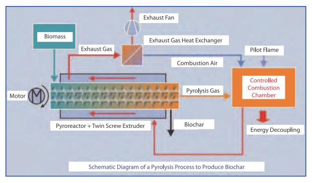
Figure 21. Scheme of a Pyrec 500 plant.
