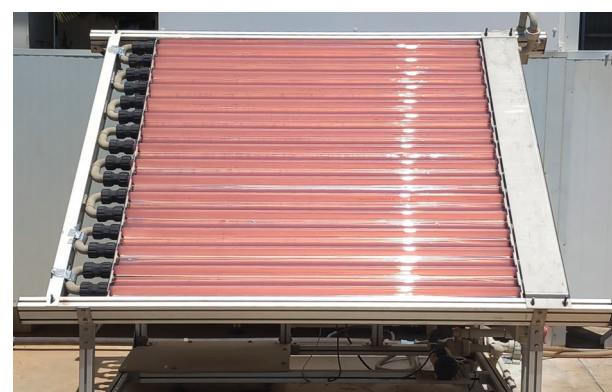
Figure 3: Solar photocatalytic pilot plant for hydrogen production Graphics: CIEMAT P.S.A
