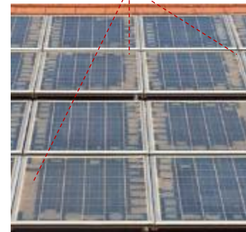
fatigue delamination (cyclic intermittent)
