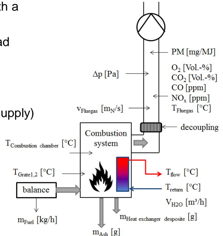
Experimental setup of combustion appliance (Figure: BE2020)
