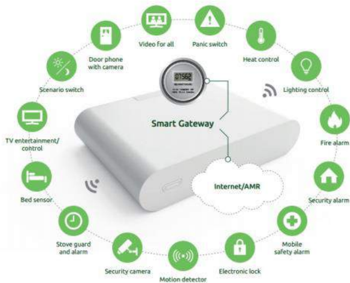
Figure 9. Lyse Energi's smart generic gateway.
