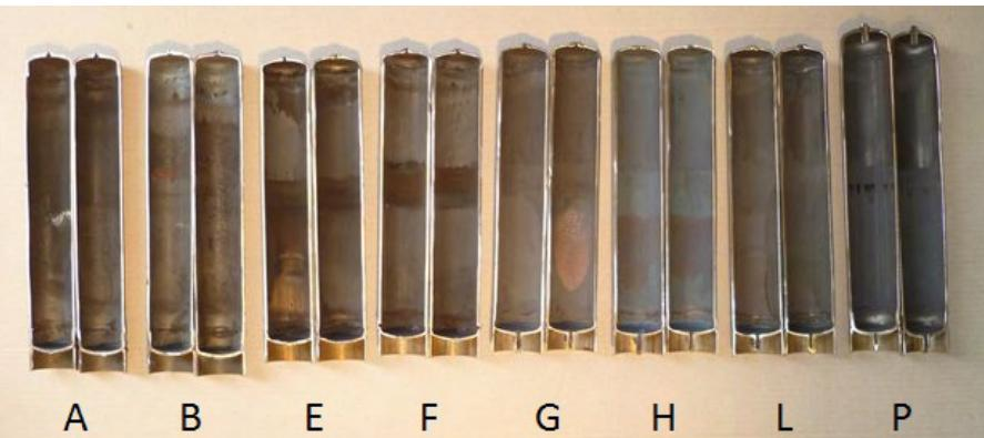
All probes show thin corrosion layer – no significant difference between probes
