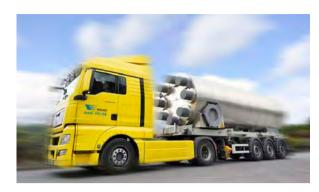
▲ Heat recuperated from a waste incinerator is transferred to an industrial drying processor using a thermo-chemical storage tank.
