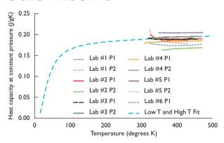
▲ Results of round-robin testing of materials samples in seven laboratories show a variance of between 4% and 9%.
