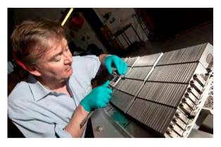
Last verification of the bulk tungsten assembly before it is installed in the remote handling unit of the Joint European Torus (JET).
