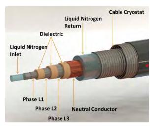
A cross-section of a high-temperature superconducting cable used in the AmpaCity project (Essen, Germany).
