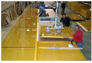
▲ Factory assembling of a large, prefabricated façade module (Austria)
