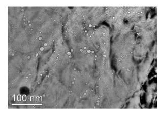
Helium bubbles in a steel specimen produced during neutron irradiation.
