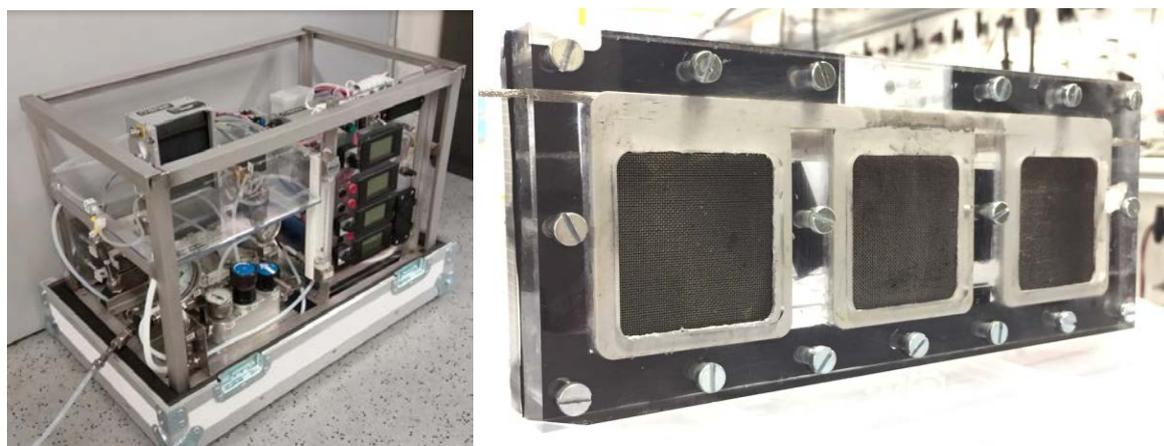
**Figure 2:** Prototypes, left: H<sub>2</sub> release reactor with PEM fuel cell, right: direct borohydride fuel cell (Source: Graz University of Technology, CEET, 2017).
