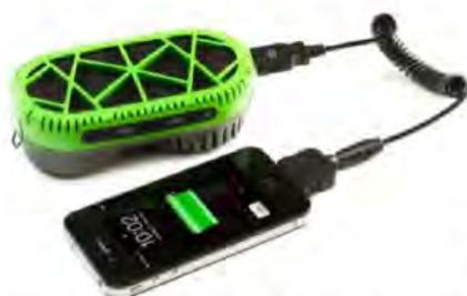
Stockholm based myFC and SiGna Chemistry have jointly launched the pocket sized hydrogen fuel cell charging power solution for mobile devices. The PowerTrek contains a sodium silicide powder, which when water is added to it at room temperature, produces enough energy to power up portable devices on the go and recharge batteries.
