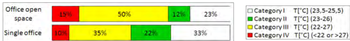
Figure 6-11. Indoor Thermal Quality expressed in percentage of time for four categories of the two analyzed rooms (Olesen et al., 2011).
