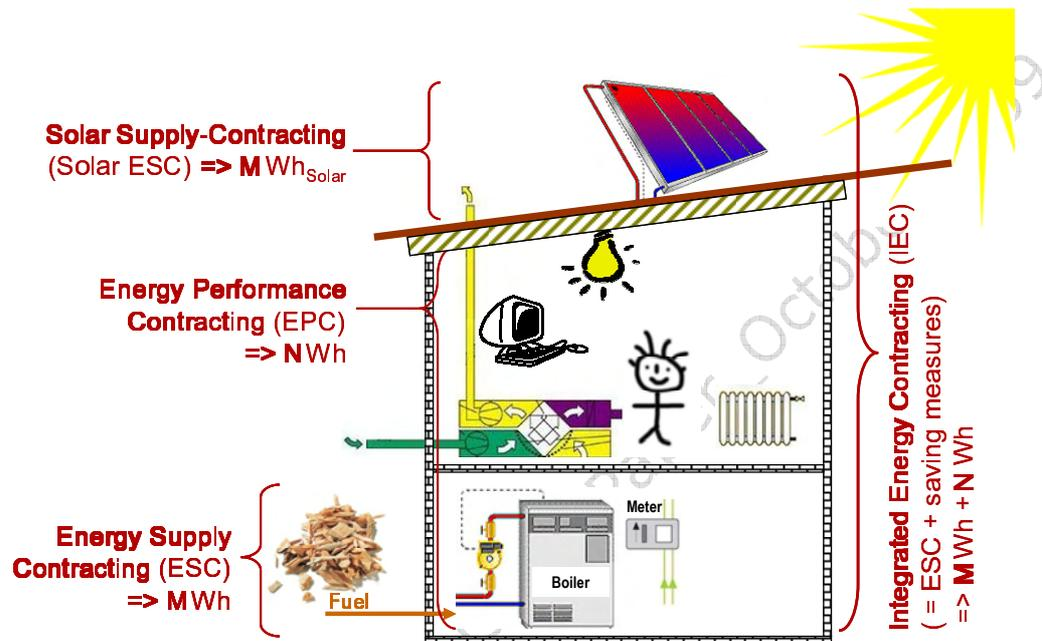
Figure 3 Scope of services of different ESCo models
