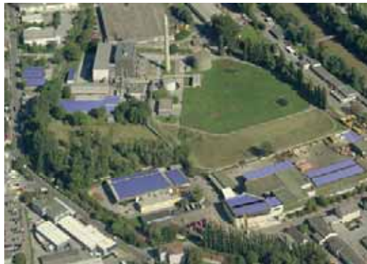
Collector area: 4062 m 2 (2008) Planned enlargement up to 6903 m 2 application of energy: about 1,800 MWh/a Commissioning: 2007-2008
