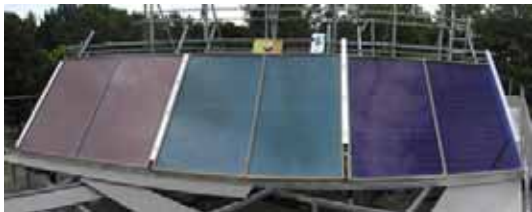
picture 31: Test rig, angle of inclination 45° (from left to right: auburn, green, selective coating of absorber), image source: [14]
