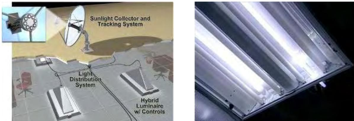
**Figure 5-27.** *HybridSolarLighting. Illustrations from Oak Ridge National Laboratory.*
