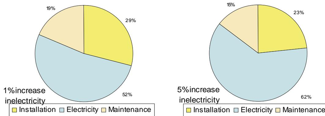
**Figure 7-10.** Distribution of costs [€/m<sup>2</sup>] for office lighting during lifecycle of an installation (24 years). Increase of 1% (left) or 5% (right) of the price of electricity has been considered.
