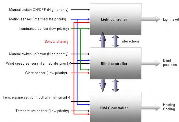
**Figure6-13.** *Interaction of the sensors on the different controller types.*
