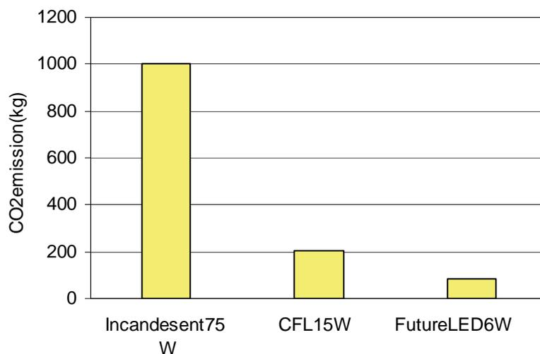
**Figure 2-9.** Comparison of CO<sub>2</sub> emissions during lifecycle (calculated for 25000 hours of time) of an incandescent lamp (12 lm/W), CFL (60 lm/W) and future LED light source (150 lm/W).
