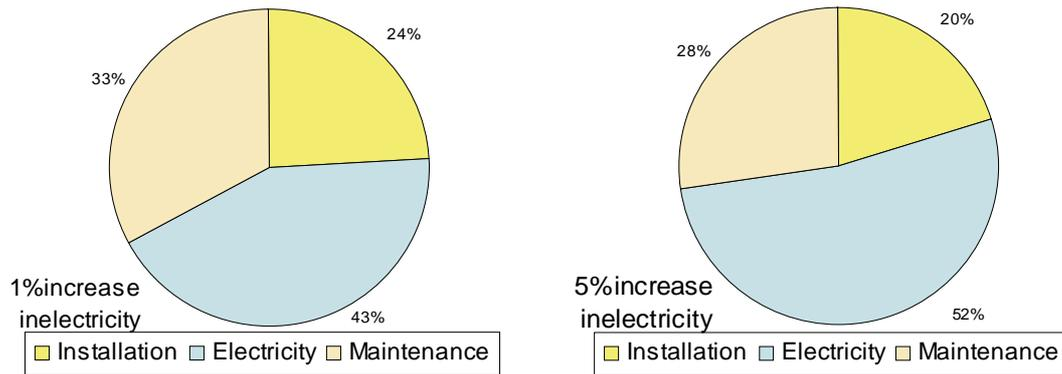
**Figure 7-9.** Distribution of costs [ $\text{€}/\text{m}^2$ ] for shop lighting during lifecycle of an installation (24 years). Increase of 1% (left) or 5% (right) of the price of electricity has been considered.
