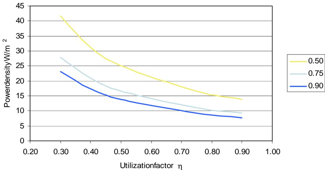
**Figure 7-5.** Power density ( $W/m^2$ ) as a function of utilization factor at different maintenance factor values ( $MF=0.50, 0.75, 0.90$ ), calculated for illuminance  $E=500lx$  and system luminous efficacy  $\eta_{\phi}=80lm/W$ .
