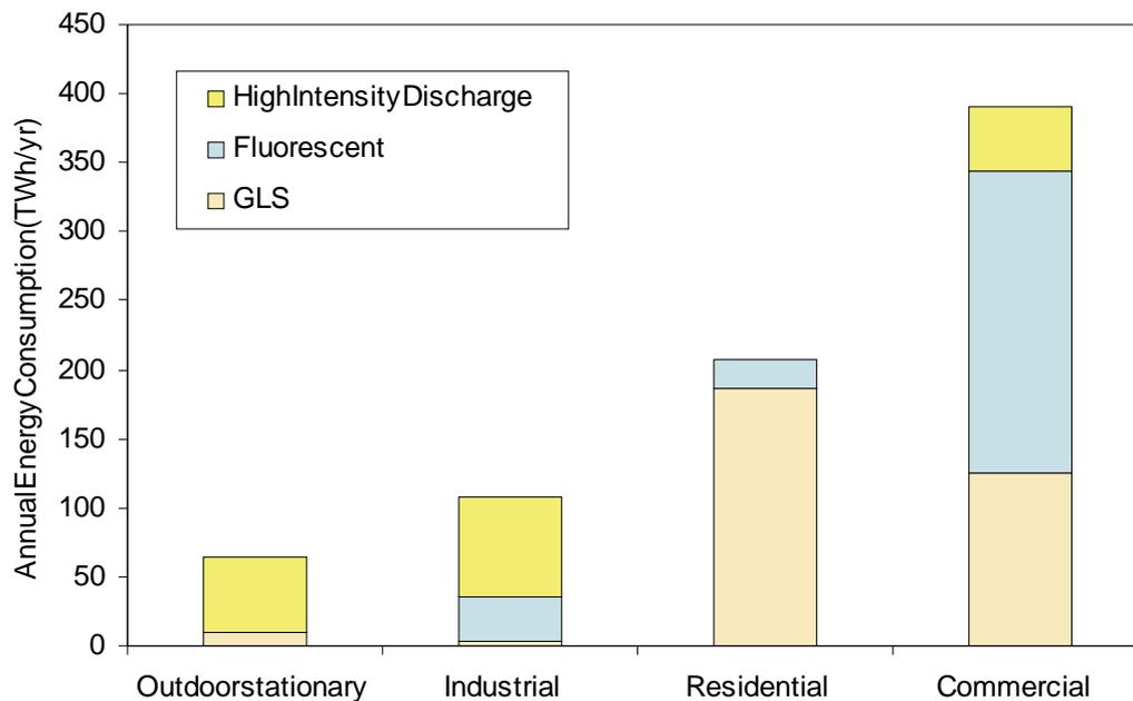
Figure 2-10. Shares of US sectoral electricity used by different light sources for lighting (Navigant 2002).
