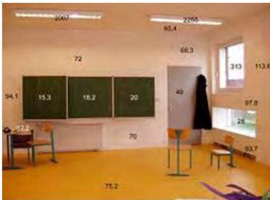
**Figure 10 -69.** Luminance measurements in north classroom.
