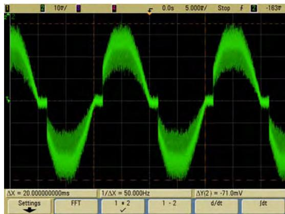
Figure5-24. Primary current waveform of an electronic transformer supplying a 50W halogen lamp.
