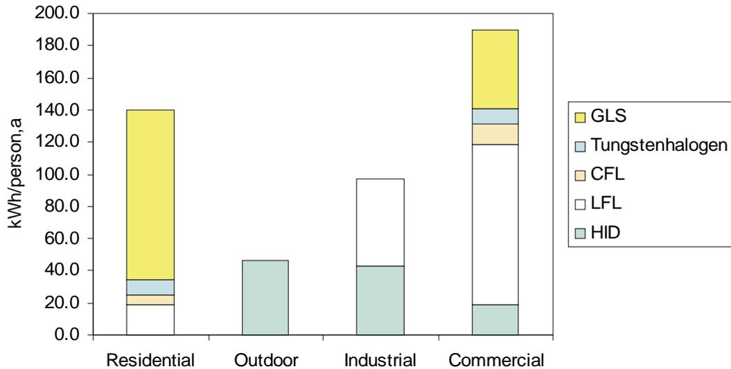
**Figure 11-2.** Estimated electric energy consumption in different sectors by lamp type in 2005. (IEA 2006)
