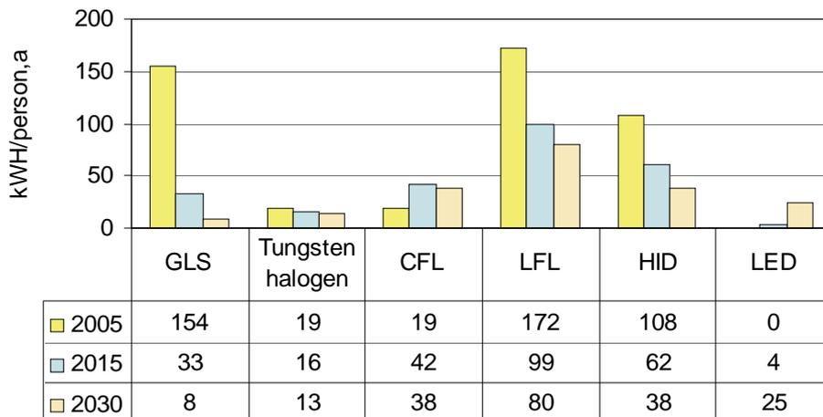
**Figure 11-6.** Status of electric energy consumption of lighting through different lamp types in 2005/2015/2030.
