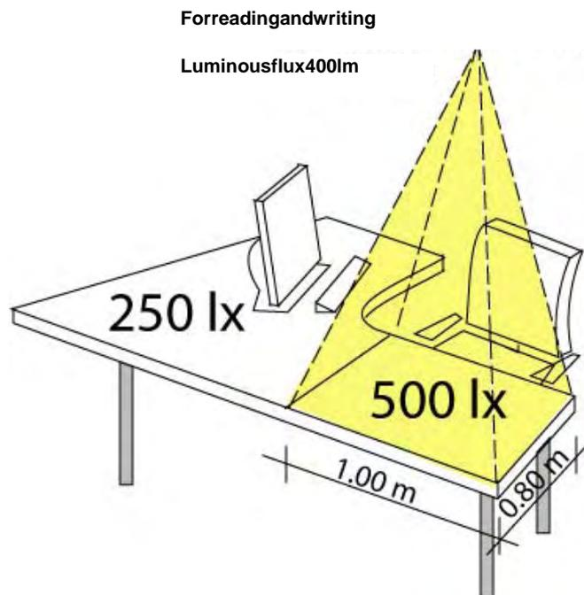
**Figure 12-1.** Possible distribution of illuminances on work plane for optimal visual performance and energy efficiency.
