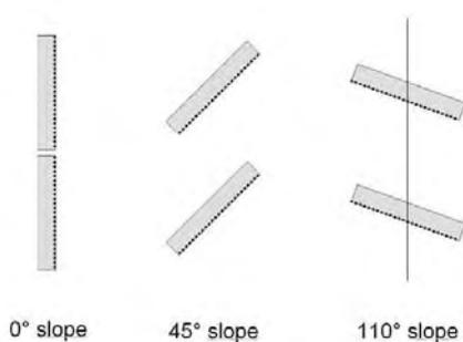
**Figure 6-42.** *Different louver positions.*
