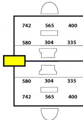
Figure 10-25. Direct-indirect stand-alone luminaire
