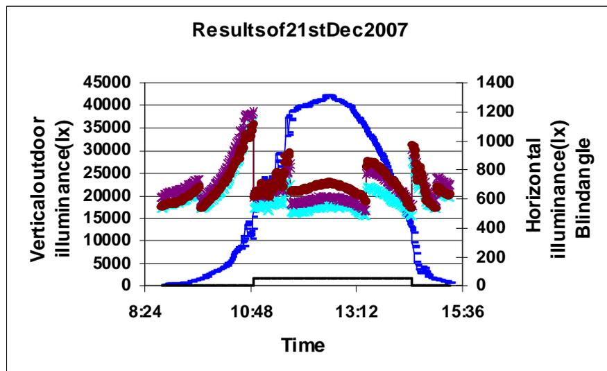
Figure 6-50. Illustration of the sensor data and operation of the blinds during one day.
