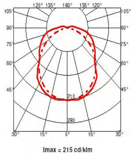
Figure10 -47. Luminairecharacteristics: Intensitydiagram.
