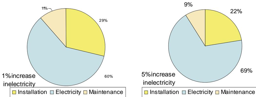
**Figure 7-11.** Distribution of costs [€/m<sup>2</sup>] for office lighting during lifecycle of an installation (24 years). Increase of 1% (left) or 5% (right) of the price of electricity has been considered. The lighting power density is 25 W/m<sup>2</sup>.
