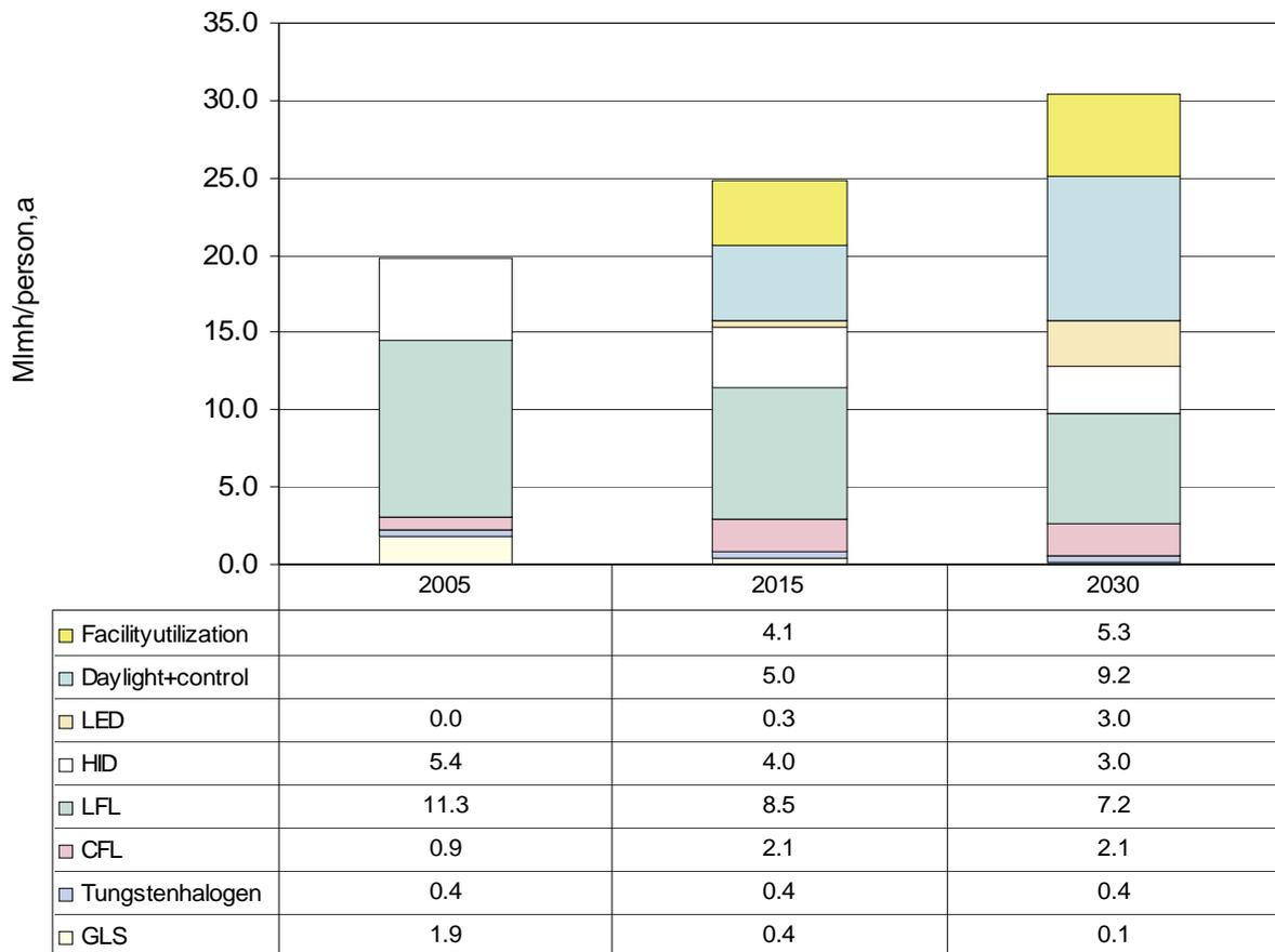
**Figure 11-5** . Development of electric light consumption through different lamp types [Mlmh/person, a] from 2005 to 2030. The facility utilization and daylight+control indicate the shares of light consumption covered by improved facility utilization and through the use of daylight and control systems.
