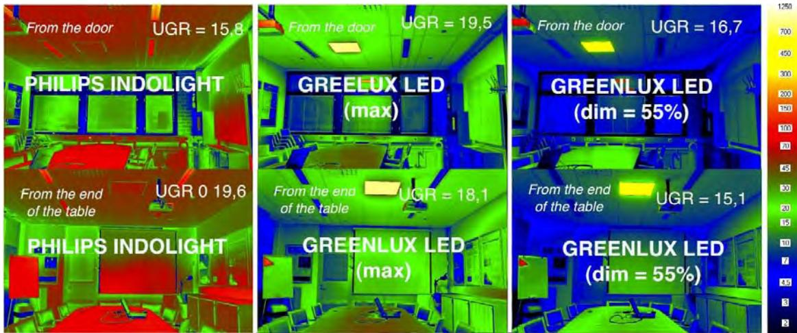
Figure 10-41. Luminance distributions of the measured room
