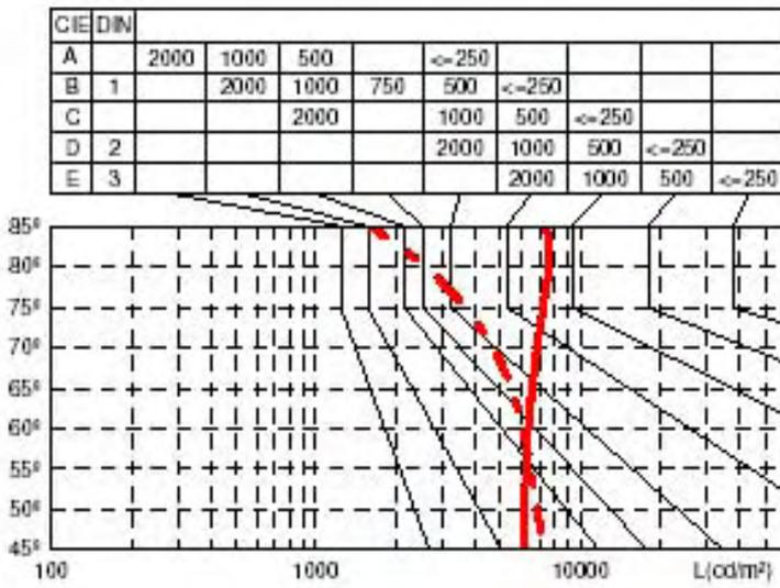
Figure 10 -46. Luminaire photometric characteristics (luminances(cd/m<sup>2</sup>)vsangles).
