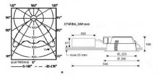
a) Photometry of the luminaire b) Geometry of the luminaire
