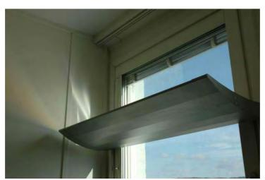
**Figure5-28.** Aprototypeofthe Daylight Luminaire. Upwardreflected sunlight as well as electrical light can be seen on the wall to the left of the luminaire.
