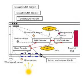
Figure 6-12. Coupling b: etween artificial lighting, daylighting and HVAC.
