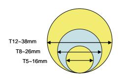
**Figure 5-4.** Comparison of tube diameter of different fluorescent lamps.
