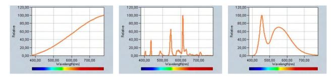
**Figure 3-3.** Light source spectrum, i.e. radiant power distribution over the visible wavelengths, determines the light color characteristics. Examples of spectra of an incandescent lamp (CCT= $2690 \, \text{K}$ , CRI=99), a compact fluorescent lamp (CCT= $2780 \, \text{K}$ , CRI=83) and awhite LED lamp (CCT= $6010 \, \text{K}$ , CRI=78).
