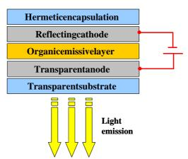
Figure 5-14. Generic structure representation of an OLED.
