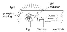
**Figure5-3.** *Operation principle of a fluorescent lamp.*
