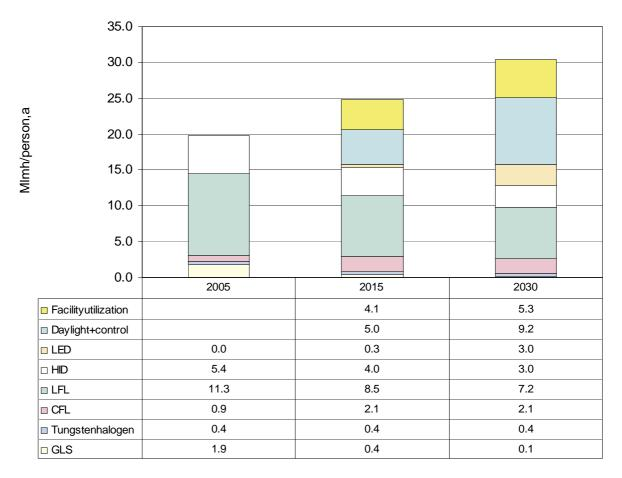
**Figure 11-5**. Development of electric light consumption through different lamp types [Mlmh/person, a] from 2005 to 2030. The facility utilization and daylight+control indicate the shares of light consumption covered by improved facility utilization and through the use of daylight and control systems.
