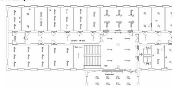
Figure 10.91 Luminaires placement (half of the 3rd floor).
