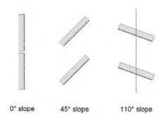
If the lamellas are located in a sunnyzone (which is function of the date and the lamella's position on the facade), they are tilted so as to be perpendicular to the rays of the sun. Their slope lies thus between 0° and 80°, in order towork as solar protection; If the plates are located in a shaded zone and if the external horizontal illumination is higher than 25.000 lx, they are placed in position of luminous penetration (slope with 110°), to work as reflectors of light.
