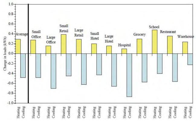
**Figure2-14.** Changesinheatingandcoolingloadscausedbya1kWhdeclineinlightingloadsinexistingUS commercialbuildings (SezganandKoomey2000).
