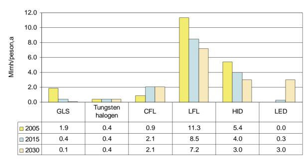
$\textbf{Figure 11-4} \ . \ \textit{Estimate delectric light consumption through different lamp types in 2005, 2015} and 2030.$
