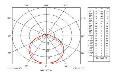
Figure 10-79. Photometry of the luminaire.
