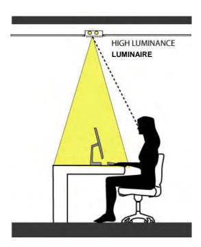
**Figure12-3.** Overheadglareissues: discomfort glareoccurs even when the luminaireis just above the occupantor, if luminaire luminance is high (above 14000 cd/m 2). Such can be the case with unshaded CFLs, LEDs, halogens and T5 fluorescent lamps.
