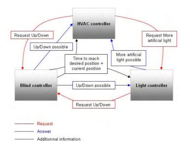
**Figure6-14.** *Example of interactions between controllers.*
