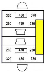
Figure 10-26. Direct-indirect suspended luminaire.
