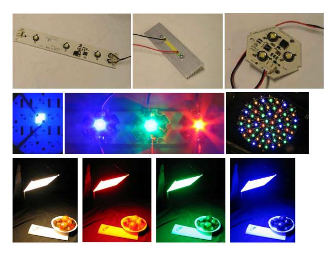
Figure 5-13. Examples of LEDs and LED modules.
