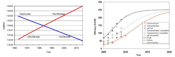
**Figure5-15.** EvolutionofthelightoutputperLEDpackage,costperlumen(left);andwhitelightLEDpackage efficacytargets(right).(DOE2010,Haitz,Kishetal.1999)
