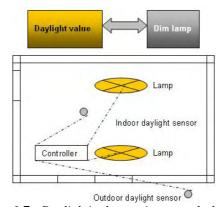
Figure 6-7. Daylighting harvesting controls cheme.
