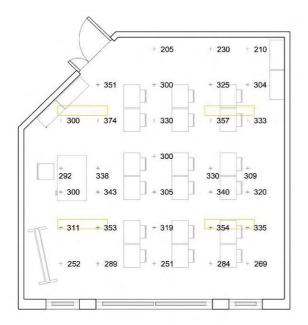
**Figure 10 - 80.** Illuminances on the work plane due to daylight: measured on 21th December at 12 am under overcast sky conditions (external illuminance 5000lx).
