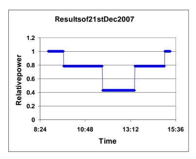
*Figure6-51. Electric power reductions during the day of Figure 6-50.*
