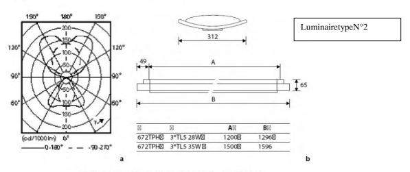
a) Photometry of the luminaire b) Geometry of the luminaire
