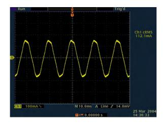
$\textbf{Figure 5-25.} \ \ \textit{Current wave form of the 20W in can descent (standard) lamp}.$
