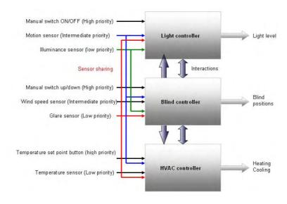
${\bf Figure 6-13.}\ {\it Interaction of the sensors on the different controller types.}$
