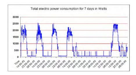
$\textbf{Figure 10-11.} \ \textit{Profile of the total power consumption of the local esduring 7 days}$
