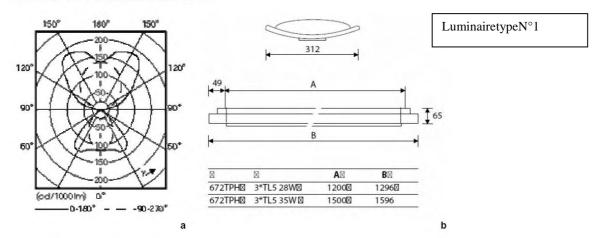
a) Photometry of the luminaire b) Geometry of the luminaire
