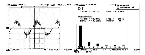
$\textbf{Figure 5-23.} \ \ \textit{Current wave form of a 0,9 WAC driven LED lamp} (20 diodes) and its spectrum.$
