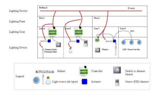
Figure 6-20. Embedded Device control.
