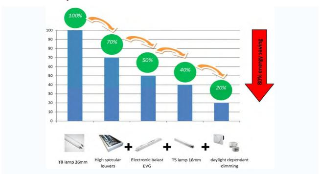
Figure 5-20. Historical development of linear fluorescent lamp luminaires regarding energy consumption.
