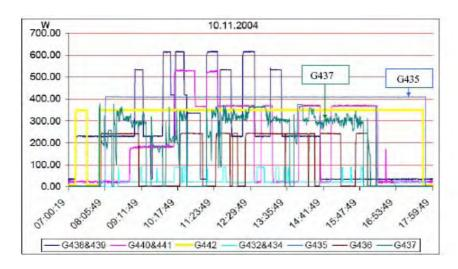
Figure 10-10 Sample of power consumption in the offices during the day
