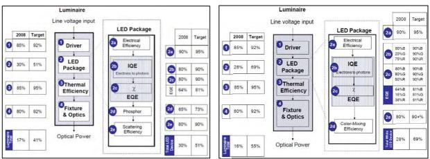
**Figure5-16.** Targetedluminaireefficienciesatsteady-stateoperationofLEDluminairescomposedofphosphor-convertedwhiteLED(left)andcolorLEDs(right). (NavigantConsultingInc.,RadcliffeAdvisorsetal.2009)
