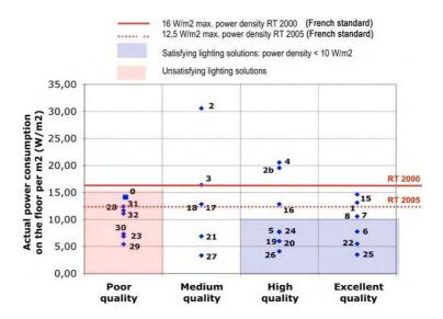
$\textbf{Figure 10-24.}\ \textit{Perceived visual quality as a function of the electric power density for lighting for 26 lighting schemes$
