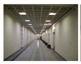
$\textbf{Figure 1 0-35.}\ 20 W tung stenhalogen lamps above the doors replaced by 2x3WR ebelLEDs.$
