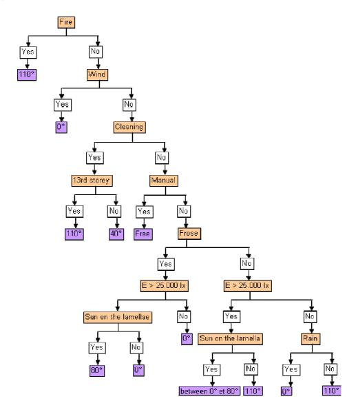
$\textbf{Figure 6-45.} \ \textit{Structure of the control strategy of the daylighting of the Berlaymont Building}.$
