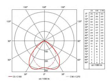
Figure 10-84. Photometry of the luminaire.
