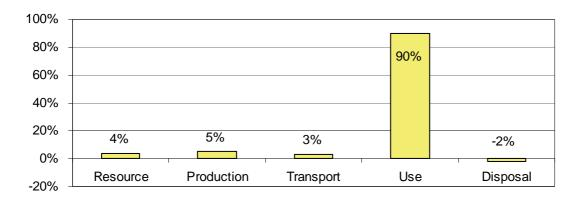
**Figure7-2.** LampenergyconsumptionduringlifecycleaccordingtoEuropeanLampCompaniesFederation(ELC 2009).
