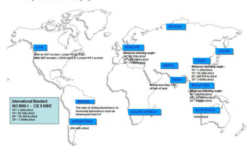
Figure 4-6. Ceilingluminances and shielding angle.
