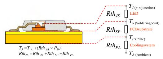
$\textbf{Figure 5-12.} \ \textit{Simplified thermal model circuit of a LED placed on a PCB}.$
