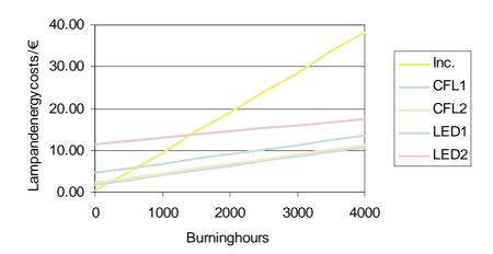
$\textbf{Figure 7-6.} \ \ Combined lamp and energy costs as a function of annual burning hours for different lamp types.$
