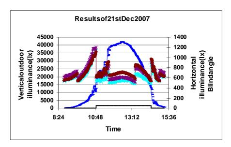
$\textbf{Figure 6-50.} \ \textit{Illustration of the sensor data} and operation of the blinds during one day.$
