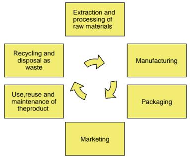
Figure 7-1. Aprinciples chematic of a life cycle analysis.
