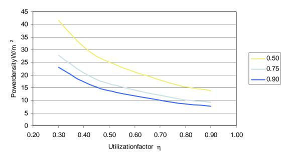
**Figure7-5.** Powerdensity(W/m $^2$ )asafunctionofutilizationfactoratdifferentmaintenancefactorvalues(MF=0.50, 0.75,0.90), calculated for illuminance E=500lx and system luminous efficacy  $\eta_{\phi}$ =80lm/W.
