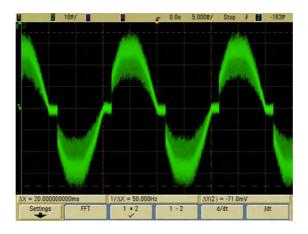
$\textbf{Figure 5-24.} \ \textit{Primary current wave form of an electronic transformer supplying a 50 Whalogen lamp.}$
