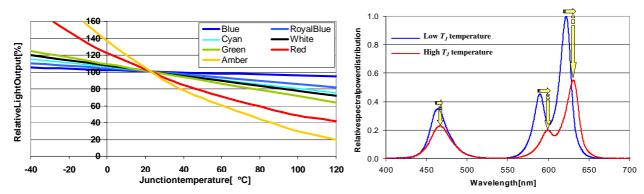
$\begin{tabular}{ll} \textbf{Figure 5-11.} & \textit{Influence of the junction temperature} (T & \textit{j}) on the light output and spectral power distribution of AlIn GaP \\ & \textit{and In GaN-based LEDs.} \end{tabular}$
