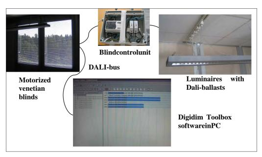
$\textbf{Figure 6-49.}\ The integrated control system interfaced to DALIbus.$
