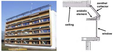
$\textbf{Figure 10-1.} \ \textit{Southern façade of the building and a cross section from the façade's system}$
