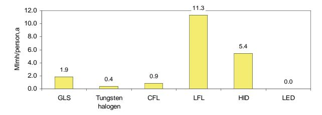
$\textbf{Figure 11-3.} \ \textit{Electric light consumption through different lamp types in 2005.} (\textit{IEA} 2006)$
