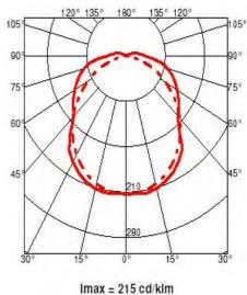
**Figure 10 - 47.** *Luminaire characteristics: Intensity* diagram.
