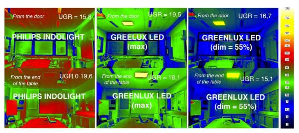
Figure 10-41. Lumin ance distributions of the measured room
