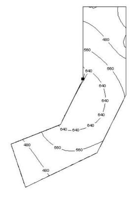
Figure 10-20. Illuminance distribution on working plane (only artificial light)
