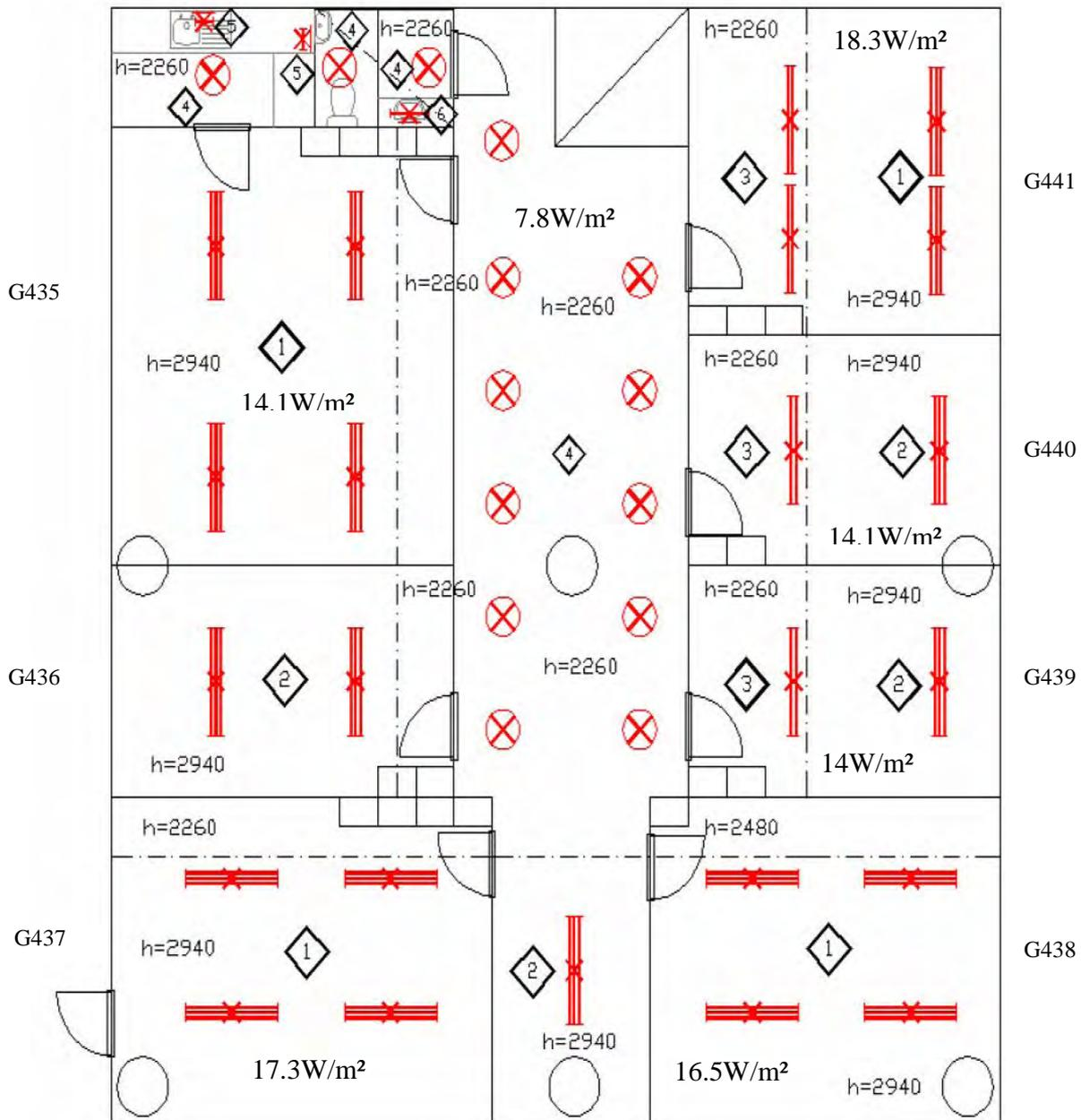
**Figure 10-5.** Office Plan with the luminaires position.
