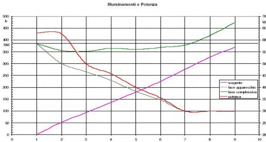
**Figure10 -49.** Exampleofdimming:dependingonanexternallightcontribution (simulating daylight), power and illuminance from the luminaire are shown. Totalilluminance(externalsourceandluminaire)isalsoshown.
