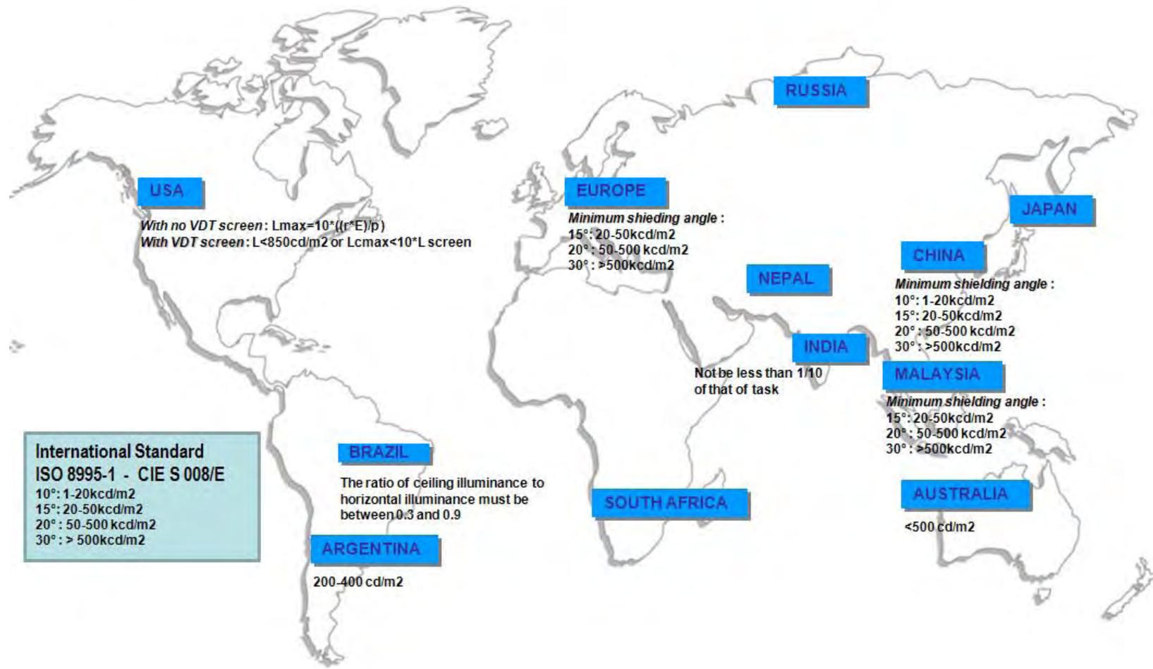
Figure 4-6. Ceiling luminances and shielding angle.
