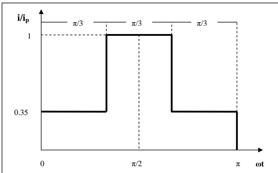
**Figure 4-8 . Limiting envelope for the current waveform.**
