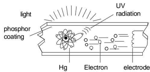
**Figure 5-3.** Operation principle of a fluorescent lamp.
