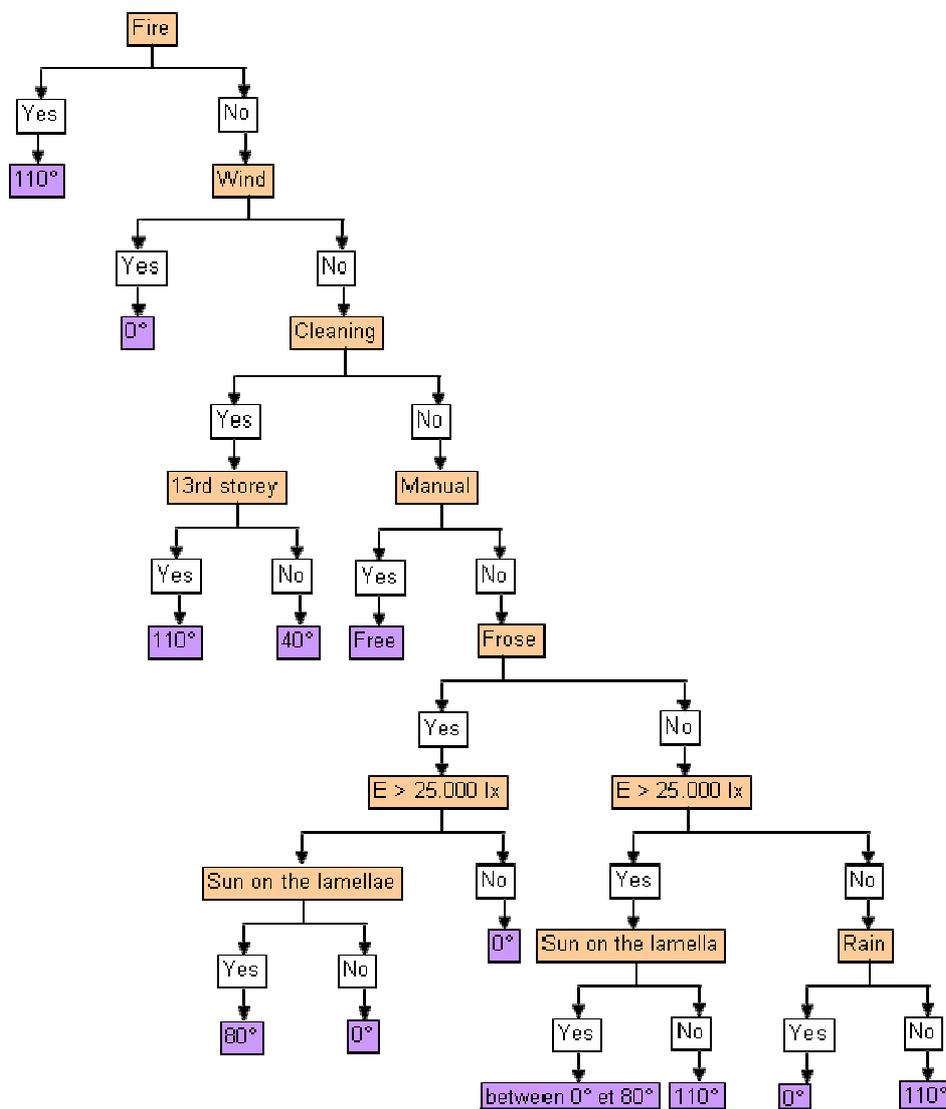
**Figure6-45.** Structure of the control strategy of the daylighting of the Berlaymont Building.
