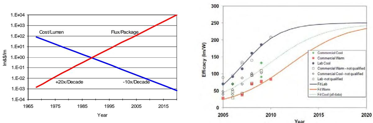
**Figure 5-15.** Evolution of the light output per LED package, cost per lumen (left); and white light LED package efficacy targets (right). (DOE 2010, Haitz, Kishi et al. 1999)
