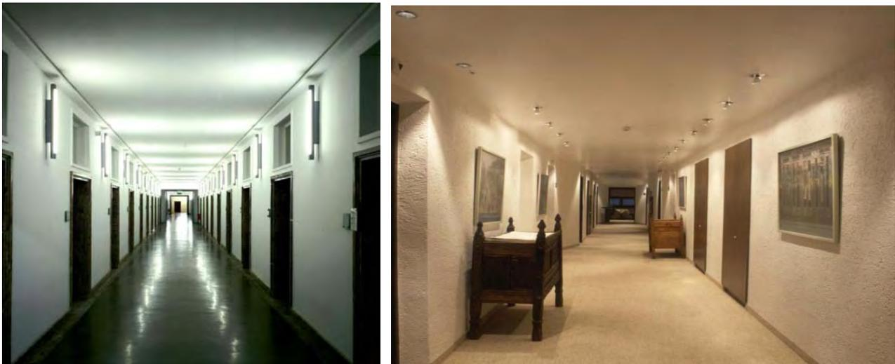
**Figure 8-4.** Comparison of two different floor lighting concepts (Bartenbach 2009).
