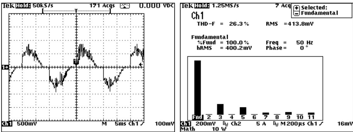
Figure5-23. Current waveform of a 0.9W AC driven LED lamp (20 diodes) and its spectrum.
