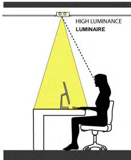
**Figure 12-3.** Overhead glare issues: discomfort glare occurs even when the luminaire is just above the occupant or, if luminaire luminance is high (above  $14000 \text{ cd/m}^2$ ). Such can be the case with unshaded CFLs, LEDs, halogens and T5 fluorescent lamps.
