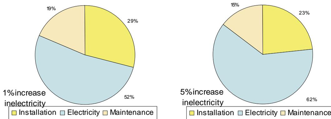
**Figure 7-10.** Distribution of costs [€/m<sup>2</sup>] for office lighting during lifecycle of an installation (24 years). Increase of 1% (left) or 5% (right) of the price of electricity has been considered.
