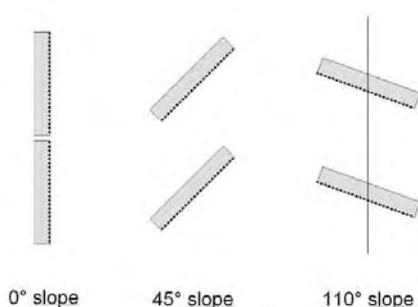
**Figure 6-42.** *Different louver positions.*
