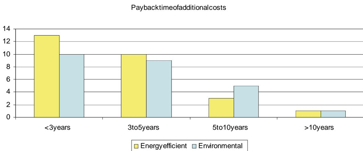
**Figure 8-12.** Payback time of additional costs of energy efficient lighting and environmental friendly technology.
