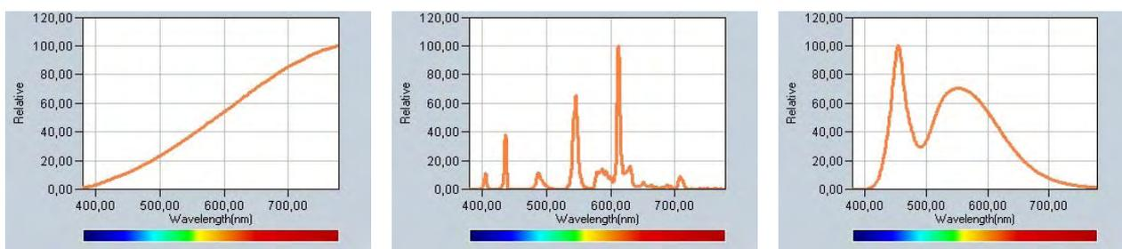
**Figure 3-3.** Light source spectrum, i.e. radiant power distribution over the visible wavelengths, determines the light color characteristics. Examples of spectra of an incandescent lamp (CCT=2690 K, CRI=99), a compact fluorescent lamp (CCT=2780 K, CRI=83) and a white LED lamp (CCT=6010 K, CRI=78).
