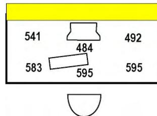
Figure 10-27. Indirect luminaire integrated in the furniture.
