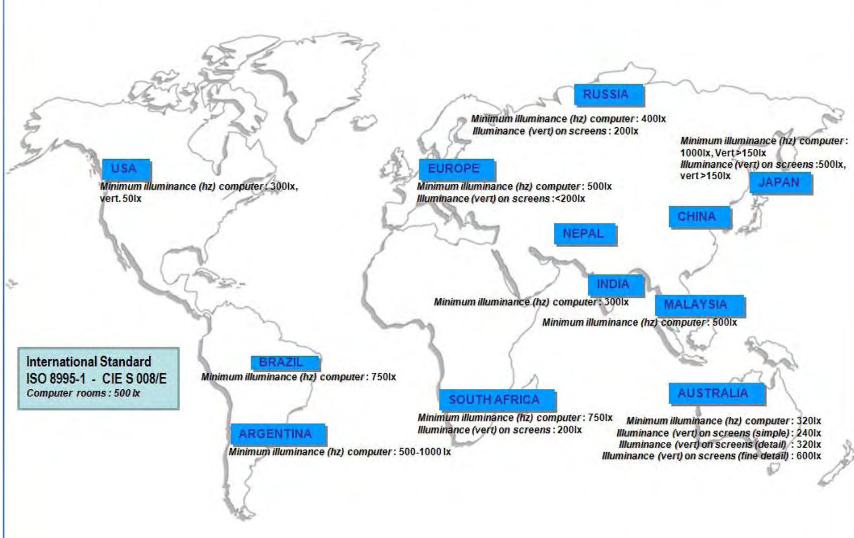
Figure4-2. Minimum illuminance on workplane for offices with computer screens.
