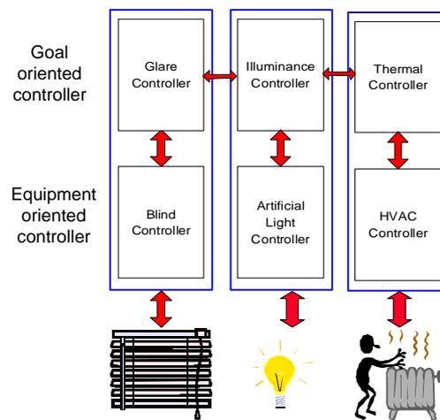
**Figure6-48.** Communication between goal oriented and equipment oriented controllers.
