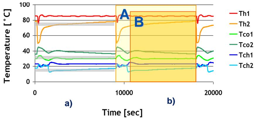
**Figure 6: Temperature profiles at generator (h), condenser (co) and evaporator (ch) of a discontinuous chiller vs. time. a) Ranges used by existing standard for the steady-state condition; b) Sub-Intervals employed in the new steady-state conditions definitions**
